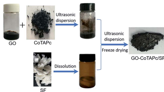
Scheme 1 Illustration for the preparation of GO-CoTAPc/SF gels.
