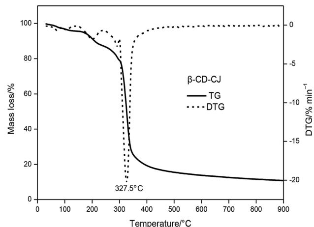
Fig. 5 TG and DTG curves of  $\beta$ -CD-CJ.
