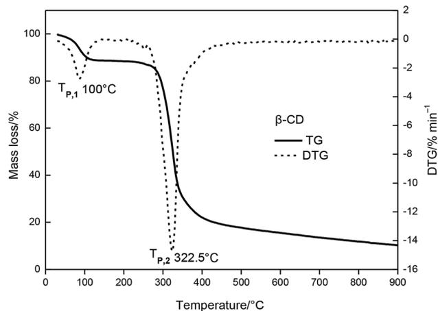
Fig. 3 TG and DTG curves of  $\beta$ -CD.
