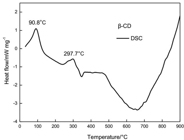
Fig. 7 DSC curve of  $\beta$ -CD.
