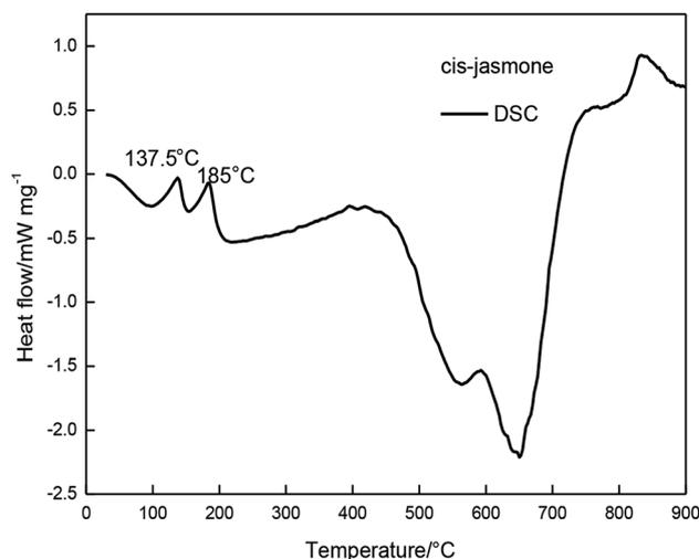
Fig. 6 DSC curve of *cis*-jasmone.
