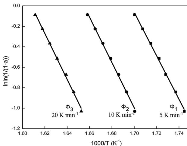
Fig. 11 The relation of  $[\ln \ln(1/(1-a))]$  and  $[1/T]$  in different heating rate.
