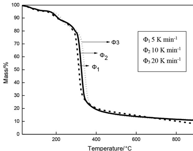
Fig. 10 TG curves of  $\beta$ -CD-CJ in different heating rate.
