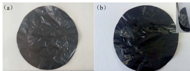
Fig. 2 Digital photographs of the nanocomposite paper (a) before and (b) after hydrothermal reduction (inset: twisted SGP showing good flexibility).
