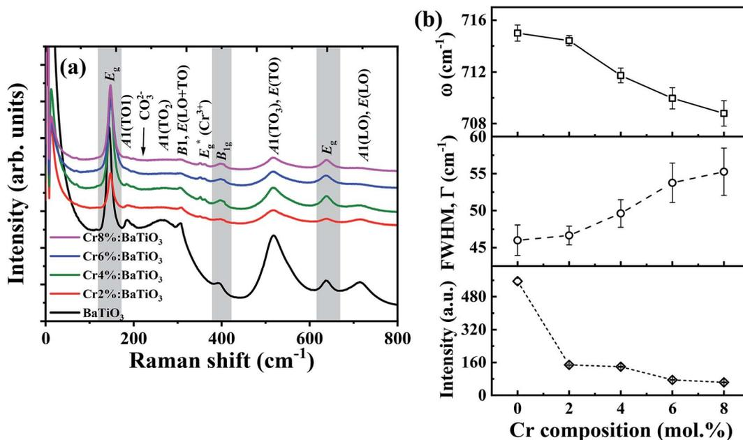
Fig. 3 (a) Raman spectra of undoped and  $\text{Cr}^{3+}$ -doped  $\text{BaTiO}_3$  lattice. Areas in ash colour indicate Raman modes of residual  $\text{TiO}_2$ . (b) Variation of phonon frequency,  $\omega$  (thick line), FWHM (dash line), and Raman intensity (short-dash line) of  $715 \text{ cm}^{-1}$  phonon mode with Cr composition. The solid lines are guide to the eye.
