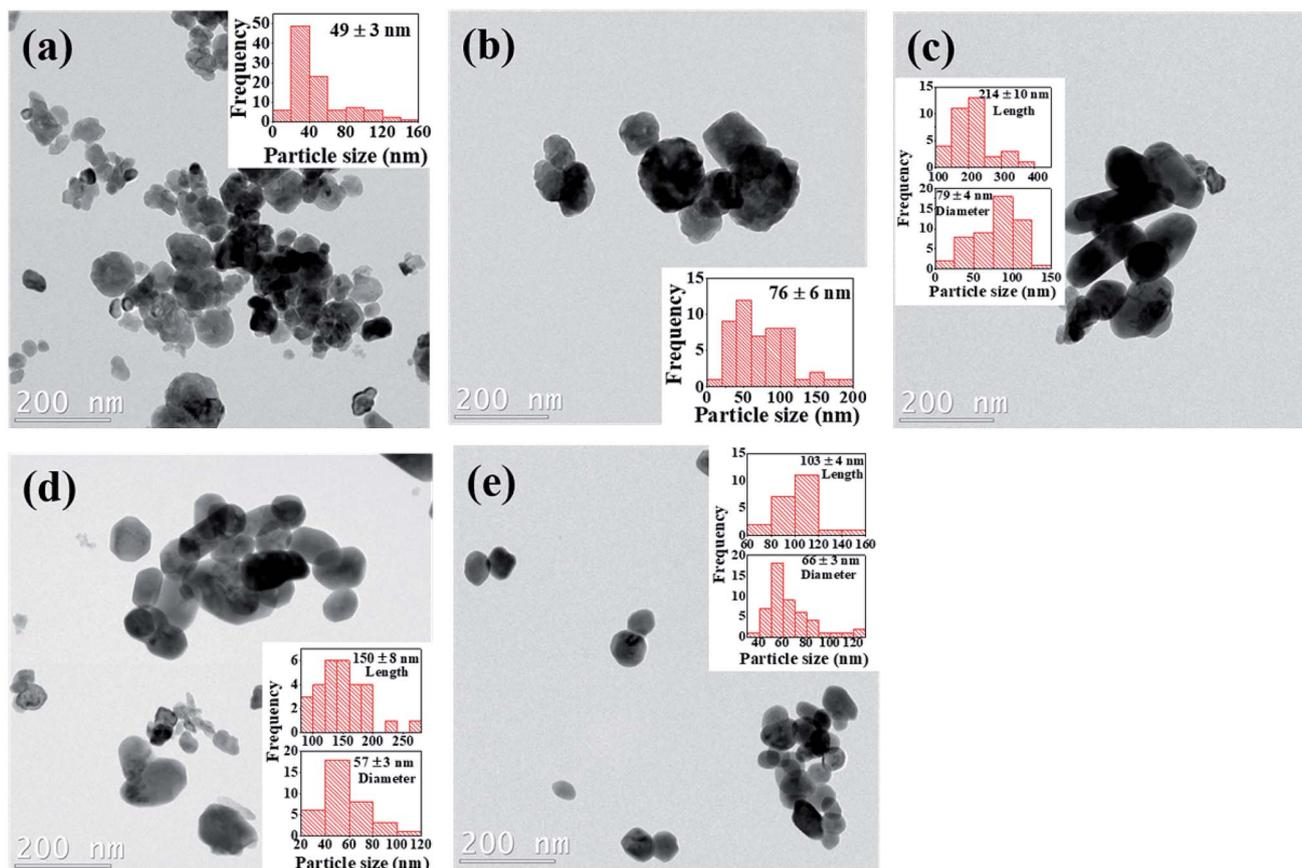
Fig. 5 Bright field TEM images of (a) undoped (b) 2 mol% Cr (c) 4 mol% Cr (d) 6 mol% Cr and (e) 8 mol% Cr<sup>3+</sup>-doped BaTiO<sub>3</sub> nanoparticles; insets are the corresponding particle size distribution.
