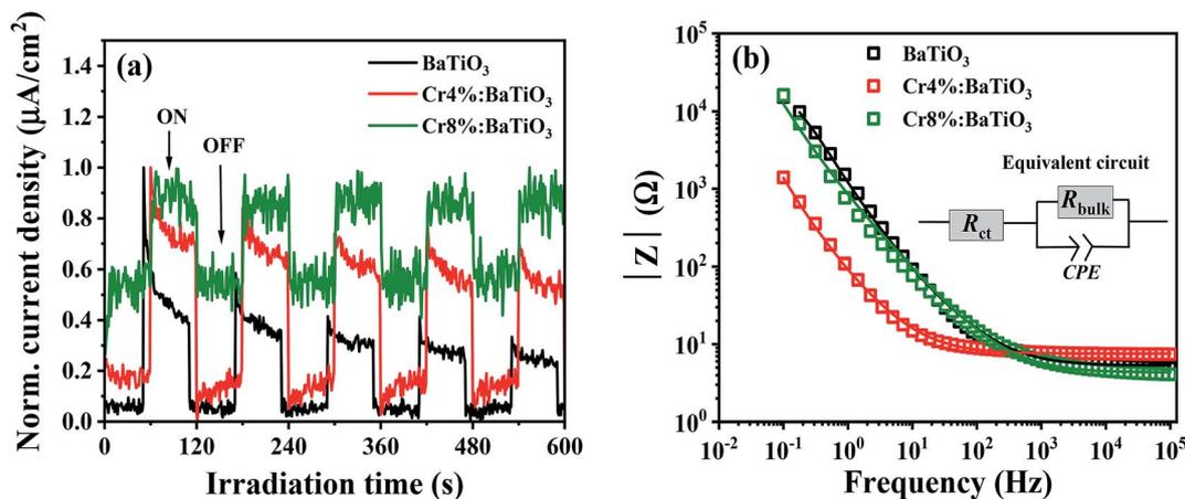
Fig. 7 (a) Normalized photocurrent density recorded at 0 V as a function of the irradiation time. (b) EIS Bode plots of the undoped (black), 4 mol% (red) and 8 mol% (green) Cr<sup>3+</sup>-doped BaTiO<sub>3</sub> samples under light irradiation.
