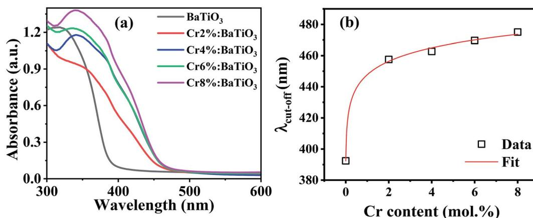
Fig. 6 (a) Optical absorption spectra of the undoped and Cr<sup>3+</sup>-doped BaTiO<sub>3</sub> samples, and (b) variation of apparent cut-off wavelength with Cr composition.
