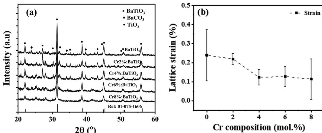
Fig. 2 (a) XRD patterns of undoped and Cr<sup>3+</sup>-doped BaTiO<sub>3</sub> nanoparticles. The peaks reflecting BaTiO<sub>3</sub>, BaCO<sub>3</sub> and TiO<sub>2</sub> are indicated by ■, ◆ and ● respectively. (b) Variation of lattice microstrain as a function Cr composition.
