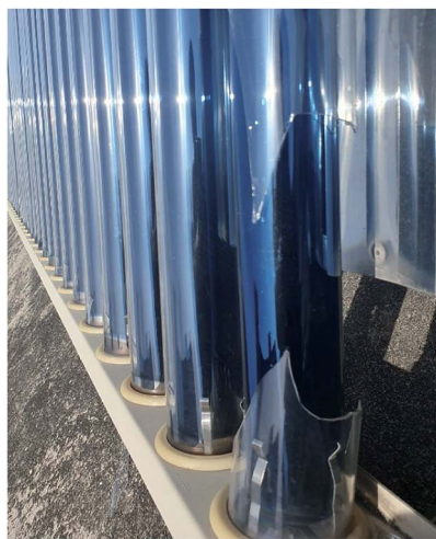
Fig. 1 Double glass tubes of ETC damaged by the impact of a small object flying in a strong wind.
