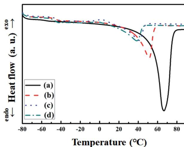
Fig. 4 DSC thermograms of (a) pure PEO, (b) intrinsic P(EO)<sub>15</sub>LiTFSI, (c) 5 wt% spherical filler-contained P(EO)<sub>15</sub>LiTFSI, and (d) 5 wt% dendritic filler-contained P(EO)<sub>15</sub>LiTFSI.
