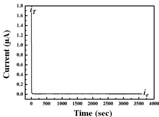
Fig. 8 Typical DC polarization curve for the cell of (stainless steel|5 wt% dendritic filler-contained P(EO)<sub>15</sub>LiTFSI|stainless steel) at 25 °C.
