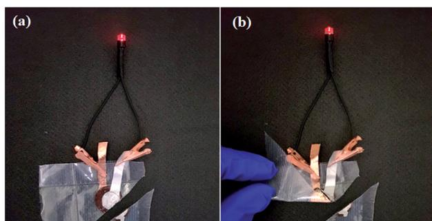
Fig. 12 Photographs of the (Li|5 wt% dendritic filler-contained P(EO)<sub>15</sub>LiTFSI|LiFePO<sub>4</sub>) pouch cell operating the LED even (a) with being cut at corner and then (b) with being folded.
