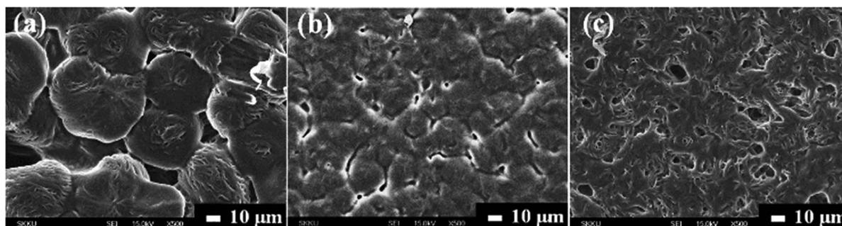
Fig. 2 Top-view FE-SEM images for (a) intrinsic  $\text{P}(\text{EO})_{15}\text{LiTFSI}$ , (b) 5 wt% spherical filler-contained  $\text{P}(\text{EO})_{15}\text{LiTFSI}$ , and (c) 5 wt% dendritic filler-contained  $\text{P}(\text{EO})_{15}\text{LiTFSI}$ .
