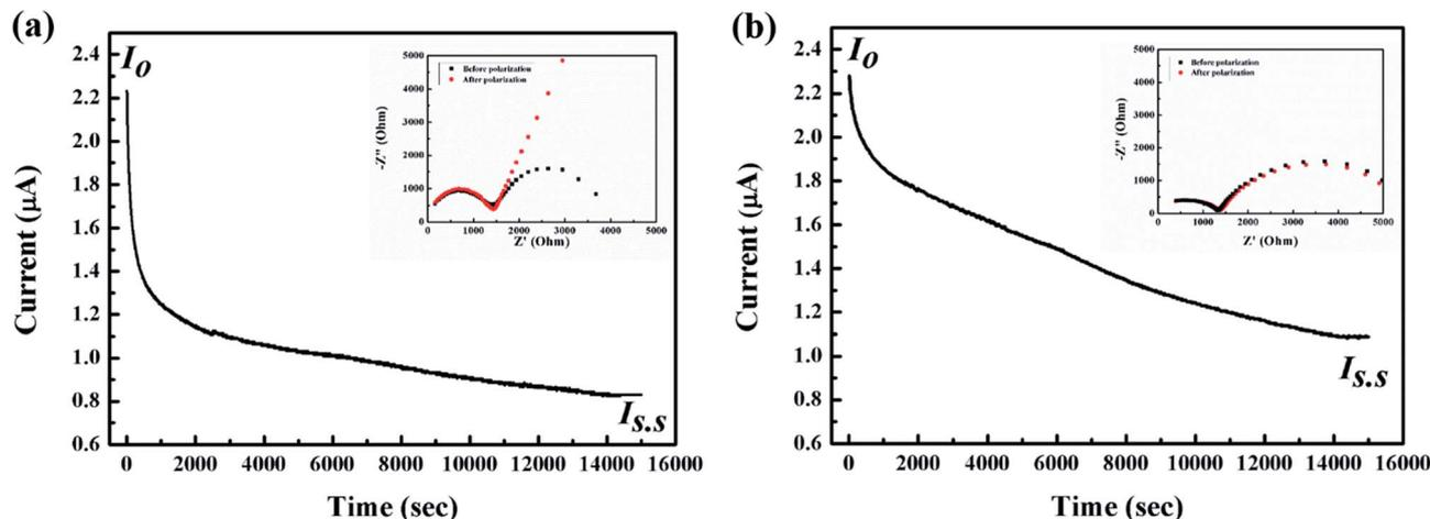
Fig. 9 Typical DC polarization curves obtained from (a) 5 wt% spherical filler-contained P(EO)<sub>15</sub>LiTFSI and (b) 5 wt% dendritic filler-contained P(EO)<sub>15</sub>LiTFSI (inset shows Nyquist plots of AC polarization before and after DC polarization at 25 °C).
