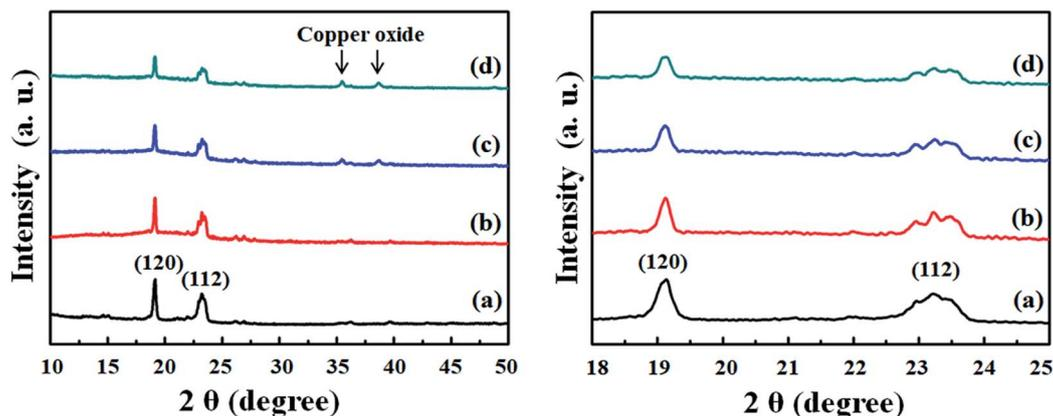
Fig. 3 XRD patterns of (a) pure PEO, (b) intrinsic P(EO)<sub>15</sub>LiTFSI, (c) 5 wt% spherical filler-contained P(EO)<sub>15</sub>LiTFSI, and (d) 5 wt% dendritic filler-contained P(EO)<sub>15</sub>LiTFSI.
