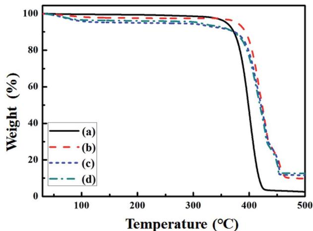
Fig. 5 TGA thermograms for (a) pure PEO, (b) intrinsic P(EO)<sub>15</sub>LiTFSI, (c) 5 wt% spherical filler-contained P(EO)<sub>15</sub>LiTFSI, and (d) 5 wt% dendritic filler-contained P(EO)<sub>15</sub>LiTFSI.
