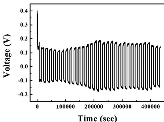
Fig. 10 Galvanostatic cycling performance of the Li symmetrical cells with 5 wt% dendritic filler-contained P(EO)<sub>15</sub>LiTFSI polymer electrolyte at a constant current density of 0.1 mA cm<sup>-2</sup>. Each half-cycle of charging and discharging step lasts 2 h at 25 °C.
