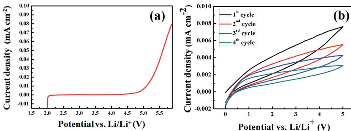
Fig. 6 (a) Linear sweep voltammetry curve and (b) cyclic voltammetry curves obtained from the cell of (Li|5 wt% dendritic filler-contained P(EO)<sub>15</sub>LiTFSI|stainless steel).
