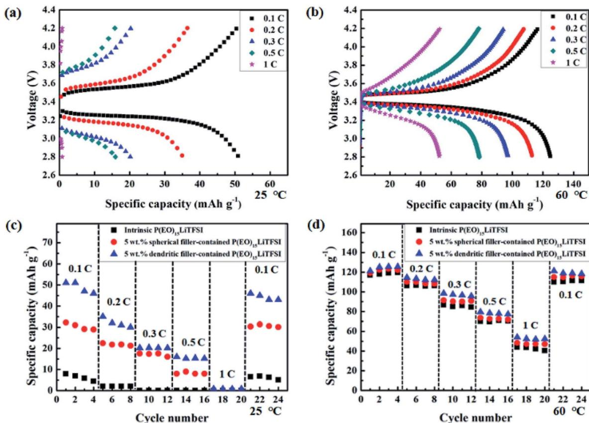
Fig. 11 The galvanic charge–discharge profiles of (Li|LiFePO<sub>4</sub>) cell using 5 wt% dendritic filler-contained P(EO)<sub>15</sub>LiTFSI with various current rates at (a) 25 °C and (b) 60 °C, and the rate performance of (Li|LiFePO<sub>4</sub>) cell with intrinsic P(EO)<sub>15</sub>LiTFSI, 5 wt% spherical filler-contained P(EO)<sub>15</sub>LiTFSI, and 5 wt% dendritic filler-contained P(EO)<sub>15</sub>LiTFSI at (c) 25 °C and (d) 60 °C.
