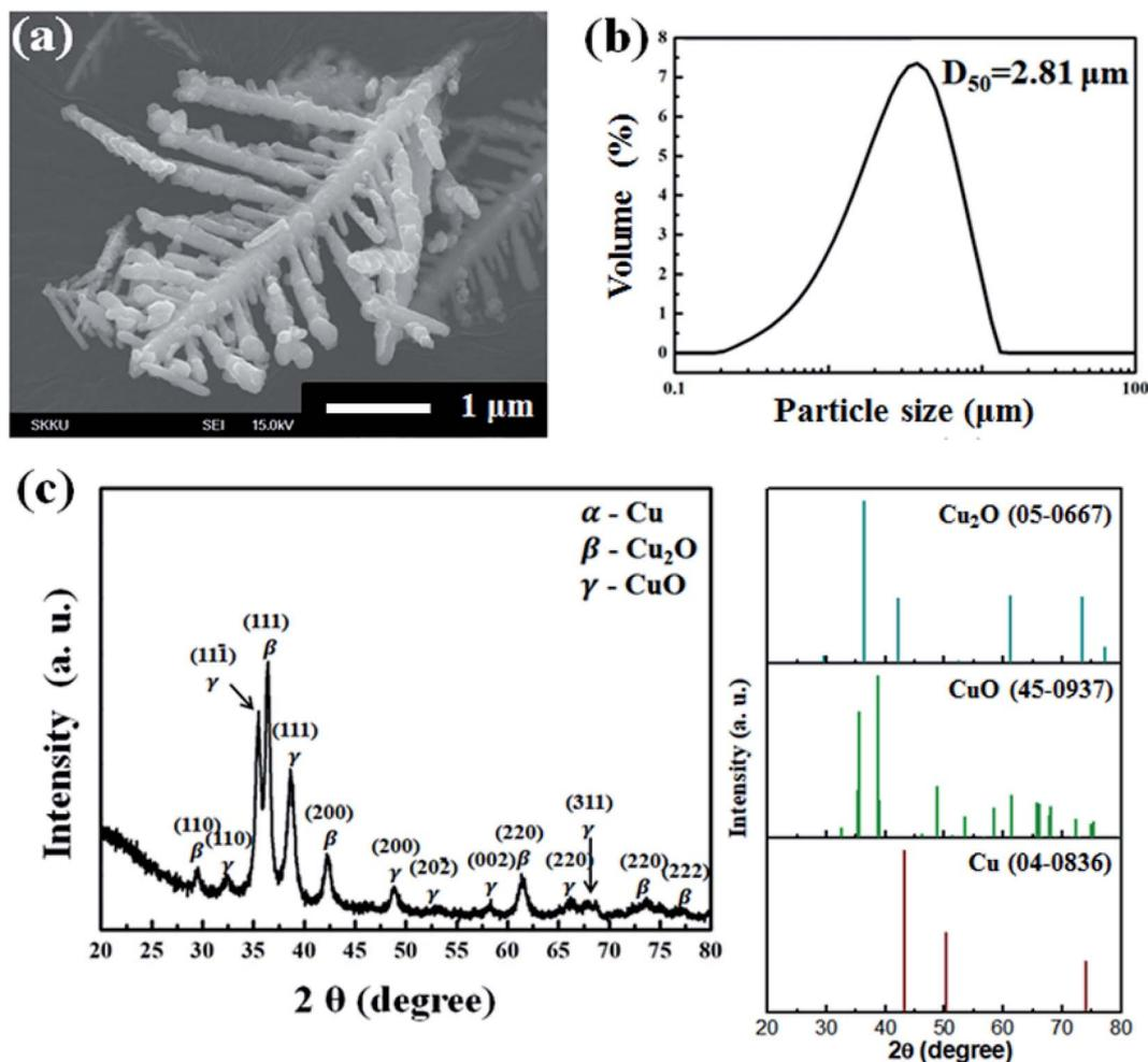
Fig. 1 Characterization of the prepared dendritic copper-oxide powders; (a) FE-SEM image, (b) the result of particle size analysis, and (c) XRD patterns.
