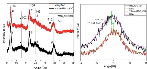
Fig. 1 XRD patterns of MoS<sub>2</sub>-rGO, and 10% V doped MoS<sub>2</sub>-rGO hybrid synthesized by modified solvothermal method. The graph at the right side is Gaussian fitting of first diffraction peaks (002) of both hybrid samples which give a clear indication of a shift in *d*-value.
