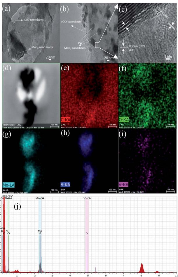
Fig. 2 TEM images of (a) MoS<sub>2</sub>-rGO (b) V doped MoS<sub>2</sub>-rGO (c) HR image of V doped MoS<sub>2</sub>-rGO. (e–i) Elemental mapping of C, O, Mo, S, and V, respectively from the region shown in (d), (j) EDX spectra of hybrid.
