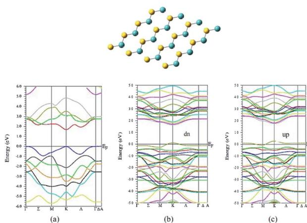
Fig. 8 Structure of MoS<sub>2</sub> and band structure for MoS<sub>2</sub> and V-doped MoS<sub>2</sub> by Veisi and coworker. (Reused with permission from ref. 49.)
