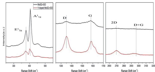
Fig. 3 Raman spectra of MoS<sub>2</sub>-rGO and V doped MoS<sub>2</sub>-rGO hybrid in three different range.
