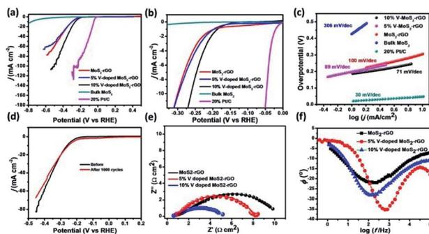
Fig. 5 (a) LSV curve for a prepared sample as well as bulk  $\text{MoS}_2$  and 20% Pt/C, (b) zoomed view of (a) at onset potential, (c) corresponding Tafel plot, (d) Stability profile for 10% V-doped  $\text{MoS}_2\text{-rGO}$  (before and after 1000 CV cycles), (e) Nyquist plot with corresponding equivalent circuit and (f) Bode plot for prepared samples.
