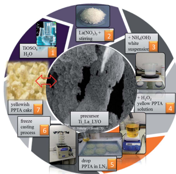
Scheme 1 Synthetic route for the preparation of [La(III)-peroxo-polytitanic Ti(IV) precursor Ti L La L LYO.
