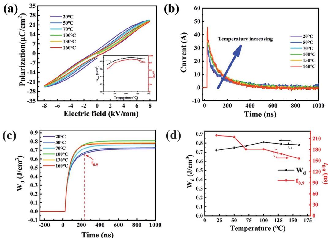
Fig. 9 (a) The temperature dependent  $P$ – $E$  loops of 5Nb ceramics at  $8 \text{ kV mm}^{-1}$ , the inset shows corresponding  $W_{\text{rec}}$  and  $\eta$ . (b) Overdamped discharging current curves of the 5Nb ceramics at  $8 \text{ kV mm}^{-1}$ . (c) The calculated  $W_d$ – $t$  curves. (d) The summarized  $W_d$  and  $t_{0.9}$  values as a function of temperature.
