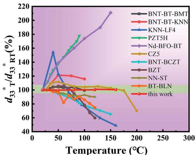
Fig. 7 Comparison of the temperature dependence of the  $d_{33}^*$  as normalized to the  $d_{33,RT}^*$  for various systems.
