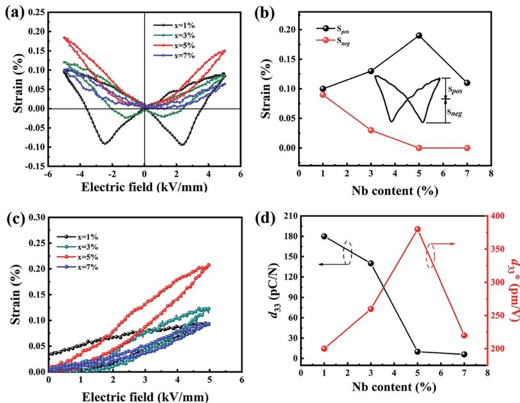
Fig. 5 The component dependent (a) bipolar strain and (c) unipolar strain curves of xNb ceramics under  $5 \text{ kV mm}^{-1}$ . (b) The evolution of component dependent  $S_{neg}$  and  $S_{pos}$ . (d) The component dependent piezoelectric constant  $d_{33}$  and normalized strain  $d_{33}^*$ .
