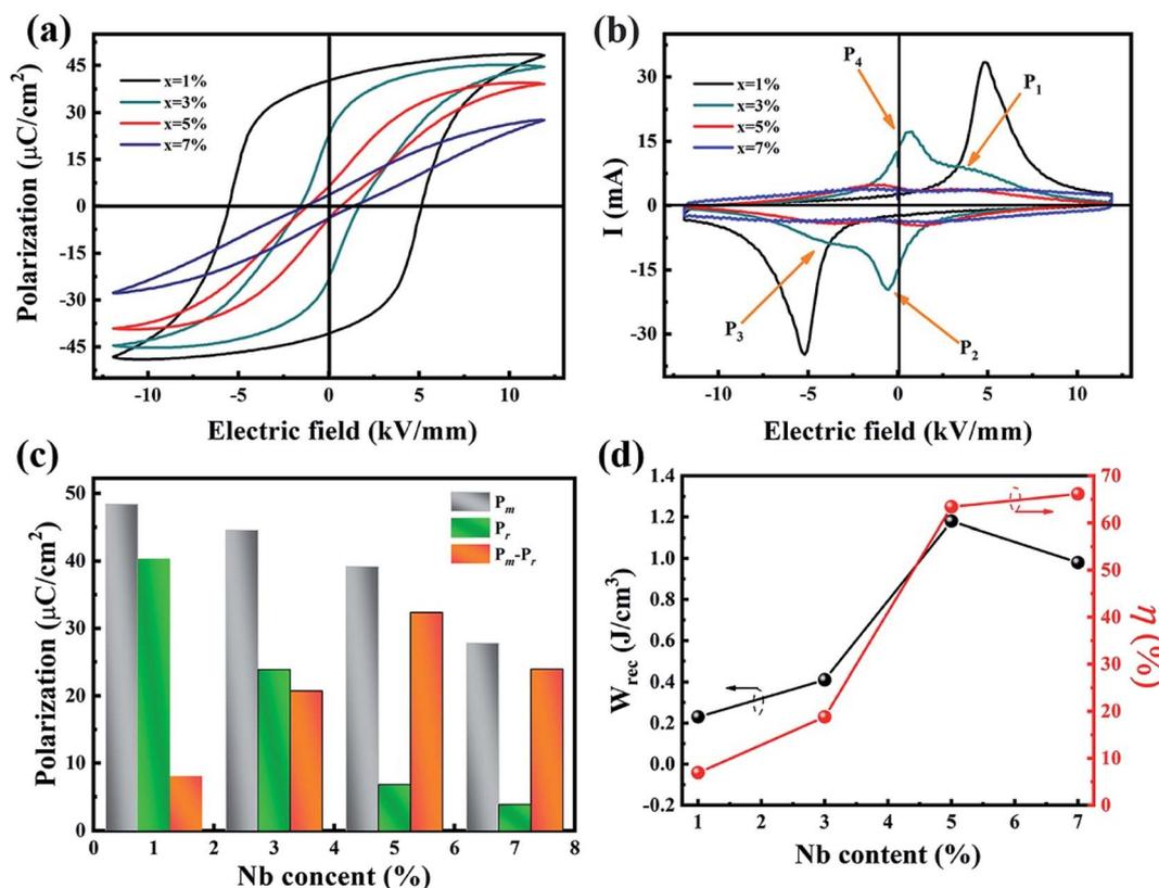
Fig. 8 (a)  $P-E$  loops of  $x\text{Nb}$  ceramics and (b) corresponding  $I-E$  curves at room temperature. (c) The component dependent  $P_m$ ,  $P_r$  and  $\Delta P (P_m - P_r)$ . (d) The component dependent calculated energy storage density and efficiency.
