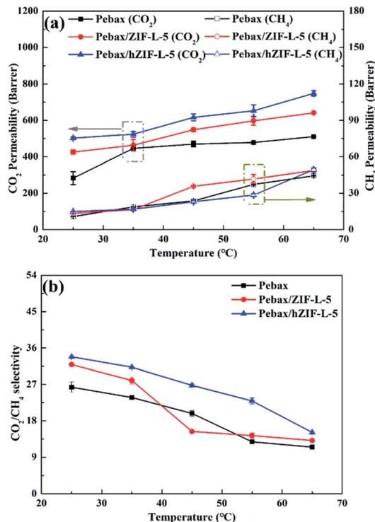
Fig. 17 Effect of operating temperature on the permeability of CO<sub>2</sub> and CH<sub>4</sub> (a) and selectivity (b).
