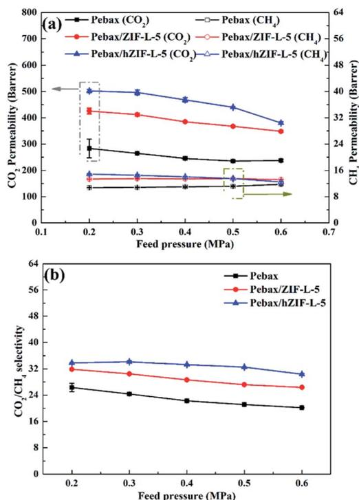
Fig. 16 Effect of feed gas pressure on the permeability of CO<sub>2</sub> and CH<sub>4</sub> (a) and selectivity (b).
