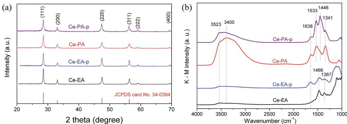
Fig. 2 XRD patterns (a) and DRIFTS spectra (b) for Ce-PA and Ce-EA as well as their precursors.
