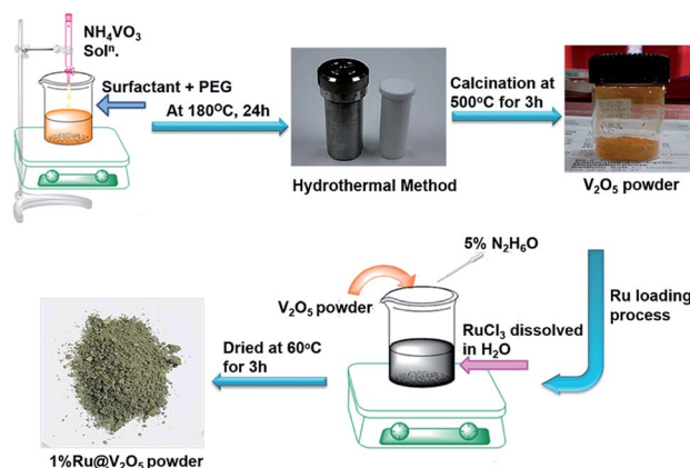
Scheme 1 Schematic representation of V_2O_5 and 1% Ru@V_2O_5 synthesis.
