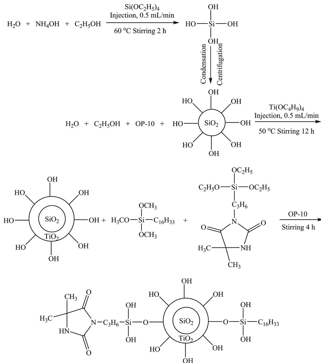
Scheme 1 Synthesis of  $\text{SiO}_2@ \text{TiO}_2$ -based core@shell composite nanoparticles.
