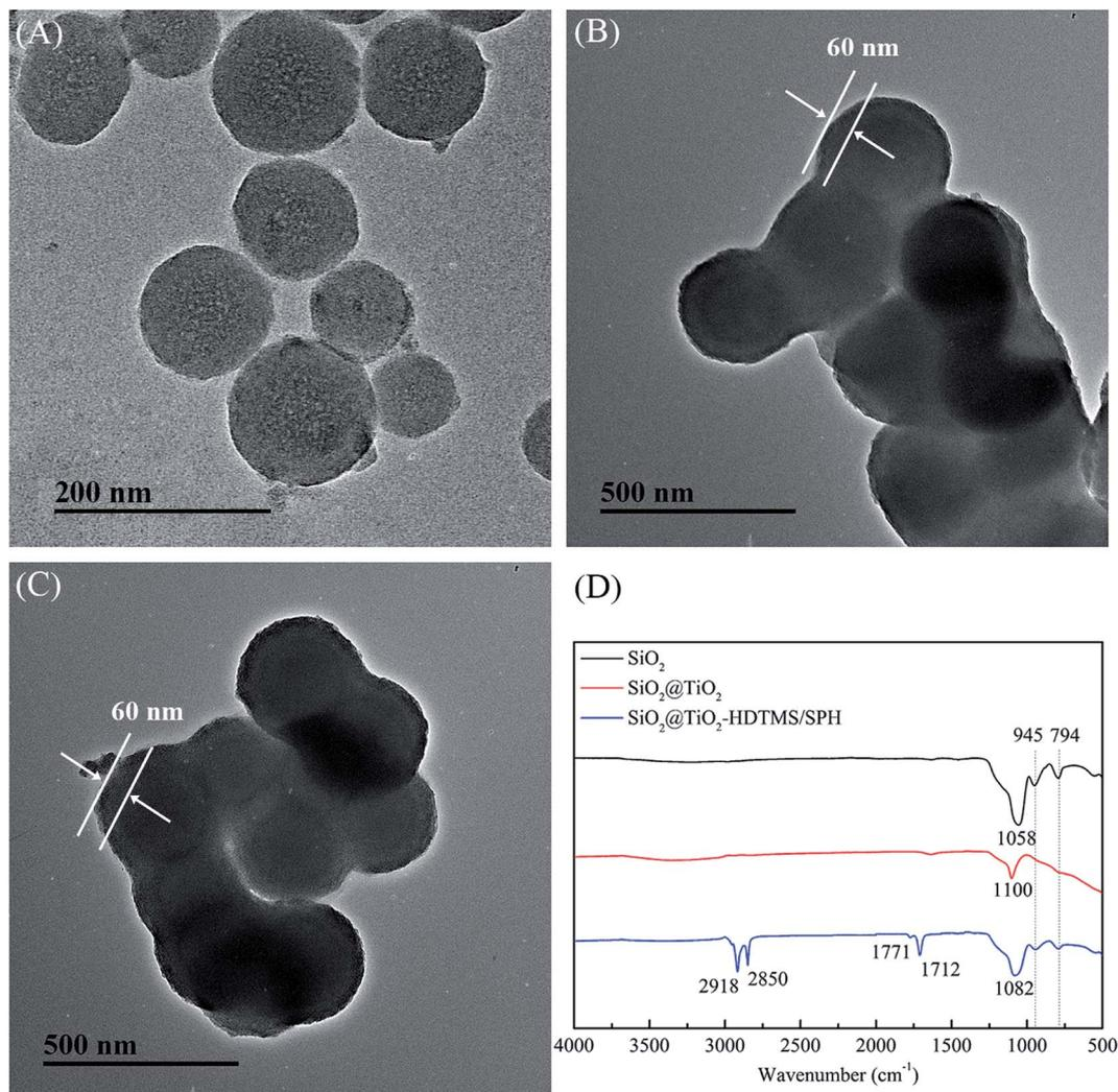
Fig. 1 TEM images of (A) SiO<sub>2</sub> NPs, (B) SiO<sub>2</sub>@TiO<sub>2</sub> NPs and (C) SiO<sub>2</sub>@TiO<sub>2</sub>-based core@shell composite nanoparticles; (D) FT-IR spectra of nanoparticles.
