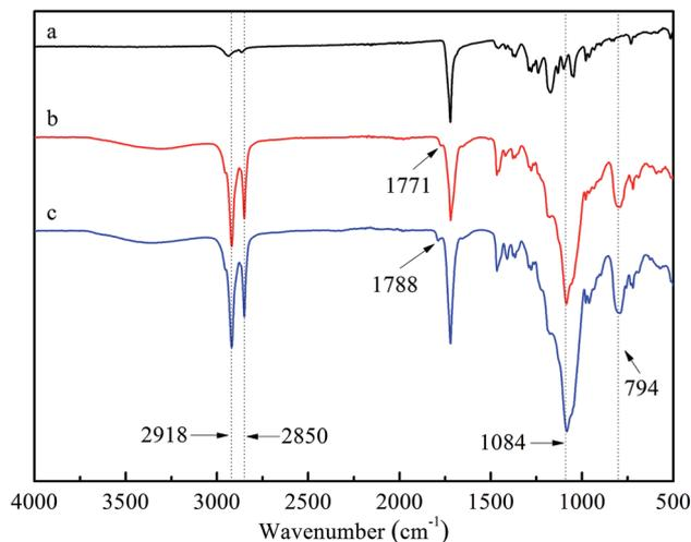
Fig. 3 FT-IR spectra of PHB/PCL (a), PHB/PCL-SiO<sub>2</sub>@TiO<sub>2</sub>-HDTMS/SPH (b) and PHB/PCL-SiO<sub>2</sub>@TiO<sub>2</sub>-HDTMS/SPH-Cl (c) fibrous membranes.
