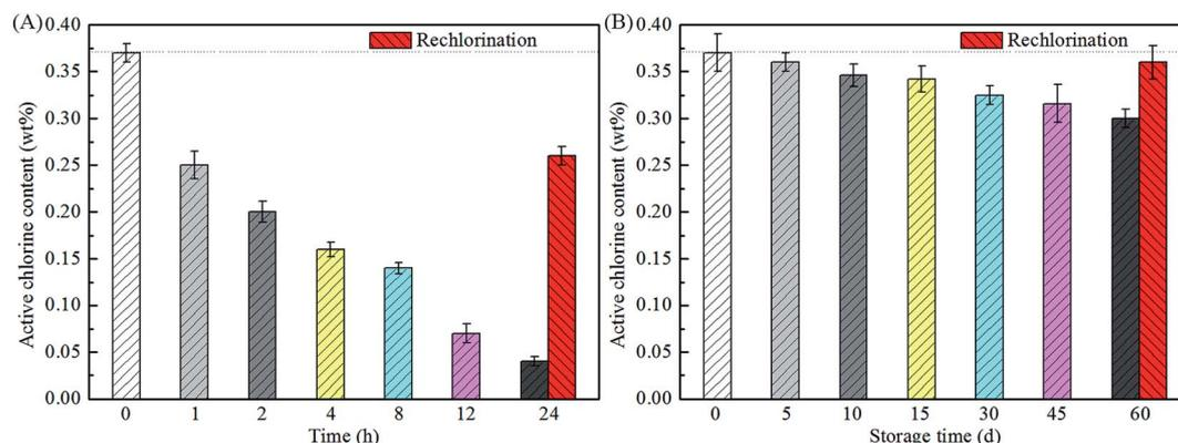
Fig. 7 UVA light stability (A) and storage stability (B) of chlorinated PHB/PCL-SiO<sub>2</sub>@TiO<sub>2</sub>-HDTMS/SPH fibrous membranes.
