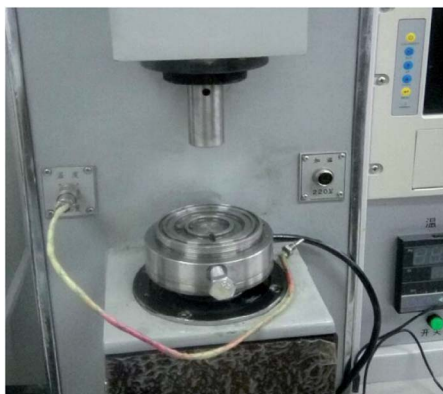
Fig. 1 MMW-1A friction and wear tester.
