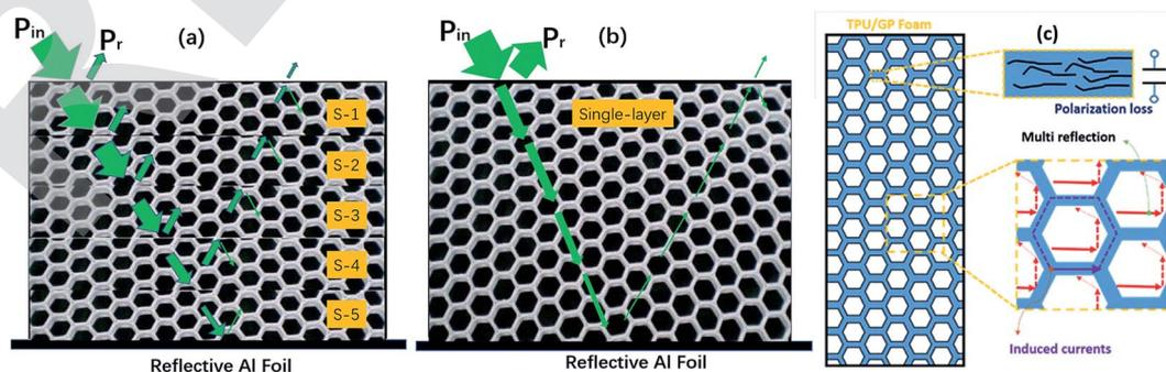
**Fig. 11** Microwave absorption mechanism diagram. (a and b) MA mechanism diagram of multilayer graphene/TPU composite foams with gradient graphene content and their corresponding single-layer sample at the same thickness. (c) MA mechanism of porous structure.
