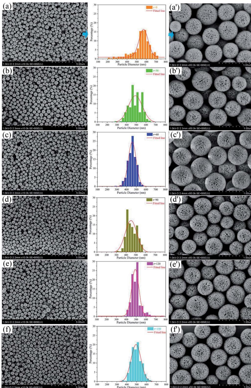
Fig. 1 SEM images with different magnifications (a–f of 5  $\mu\text{m}$  as well as a'–f' of 1  $\mu\text{m}$ ) and diameter distribution curves of KCC-1 synthesized by a facile one-pot rotating hydrothermal approach with different stirring rates of 0 (a–a'), 30 (b–b'), 60 (c–c'), 90 (d–d'), 120 (e–e'), 120 (e–e'), and 150 rpm (f–f'), respectively.
