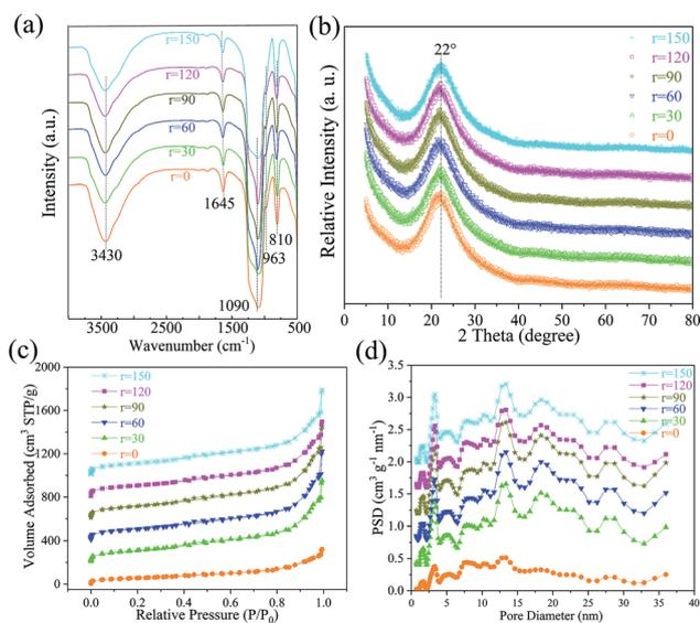
Fig. 4 FT-IR (a), XRD (b),  $N_2$  adsorption–desorption isotherms (c), and their corresponding pore size distributions (d) of KCC-1 synthesized by a facile one-pot rotating hydrothermal approach with different stirring rates of 0, 30, 60, 90, 120, and 150 rpm, respectively. Note: each curve of a higher stirring rate shifts  $200 \text{ cm}^3 \text{ STP g}^{-1}$  and  $0.4 \text{ cm}^3 \text{ g}^{-1} \text{ nm}^{-1}$  upward in Fig. 3c and d, respectively.
