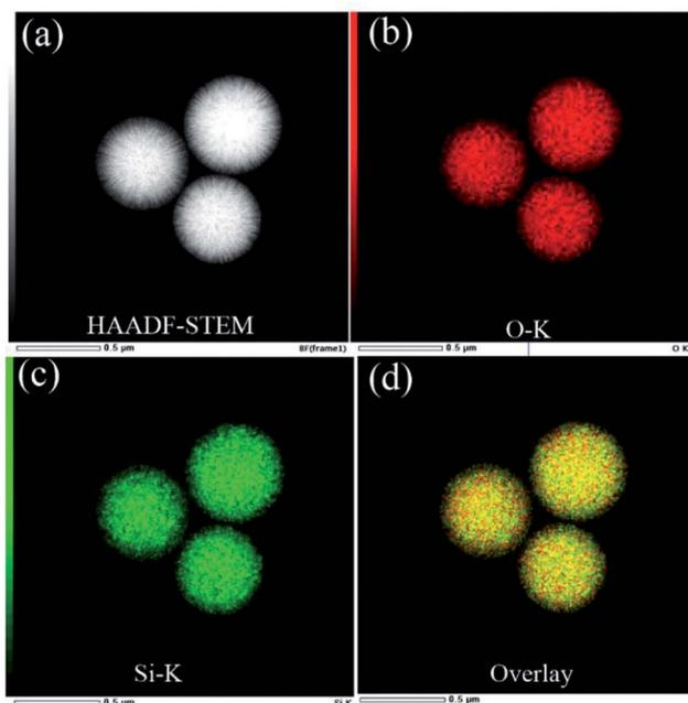
Fig. 3 STEM-EDS mapping of KCC-1 prepared at 60 rpm. FT-IR, XRD,  $N_2$  adsorption–desorption isotherms analyses.
