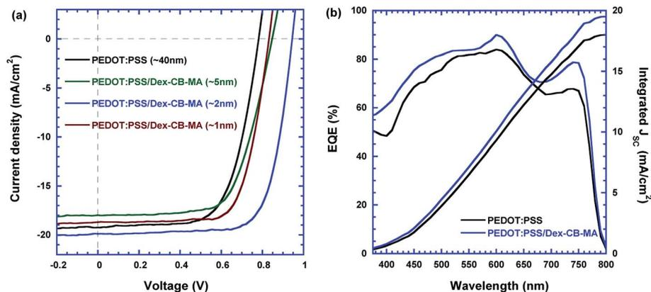
Fig. 3 (a) The  $J$ - $V$  characteristics of perovskite solar cells with different hole extraction layers (HEL), and (b) the EQE spectra of perovskite solar cells with the PEDOT:PSS HEL and the PEDOT:PSS/Dex-CB-MA HEL.
