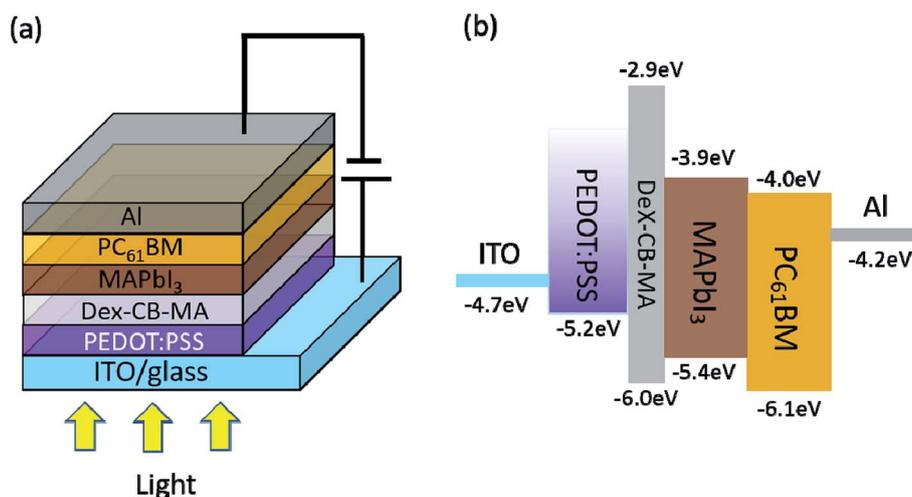
Scheme 1 (a) The device structure of perovskite solar cells, and (b) the LUMO and HOMO energy levels of Dex-CB-MA,  $\text{CH}_3\text{NH}_3\text{PbI}_3$ ,  $\text{PC}_{61}\text{BM}$ , and the work functions of ITO, PEDOT:PSS and Al.
