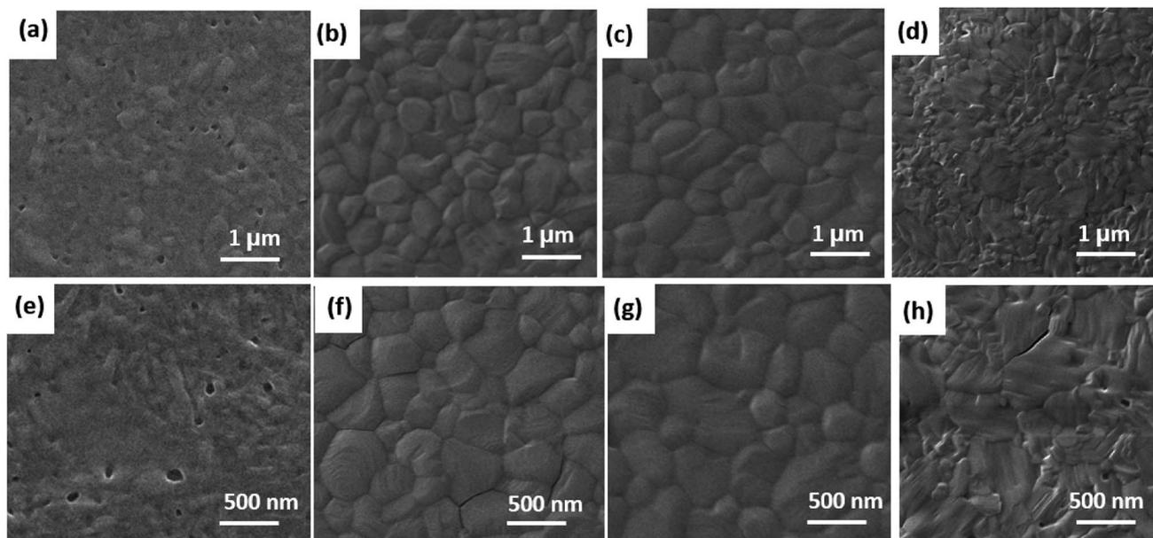
Fig. 4 The top-view SEM images of  $\text{CH}_3\text{NH}_3\text{PbI}_3$  thin films on the top of different thickness of Dex-CB-MA thin layer, (a) and (e) 0 nm, (b) and (f) 1 nm, (c) and (g) 2 nm, (d) and (h) 5 nm. The top images are by 50k times and the bottom images are by 100k times, respectively.
