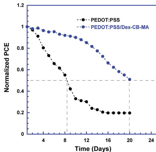
Fig. 7 Self-stability of PSCs with the PEDOT:PSS HEL and the PEDOT:PSS/Dex-CB-MA HEL, respectively.
