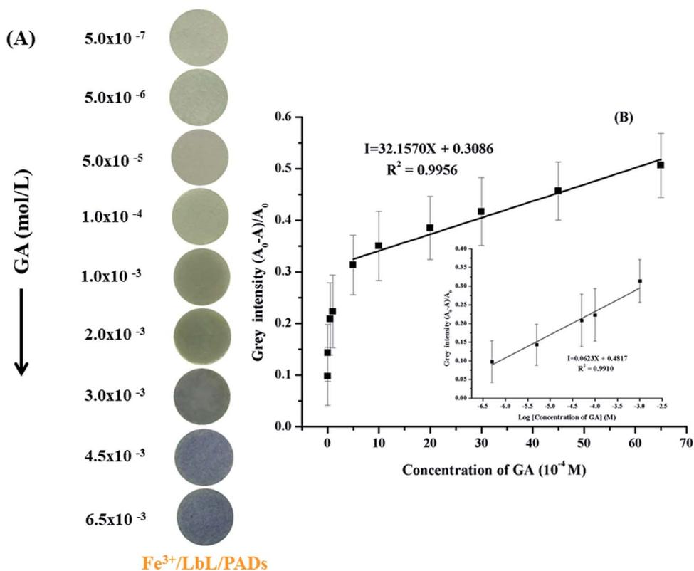
Fig. 7 (A) Photographic images of the  $\text{Fe}^{3+}/(\text{TBABr}/\text{SDS})_3/\text{PAD}$  sensor color changes at various concentrations of GA. (B) Plot of grey intensity of  $\text{Fe}^{3+}/(\text{TBABr}/\text{SDS})_3/\text{PAD}$  sensor as a function of the concentration of GA.
