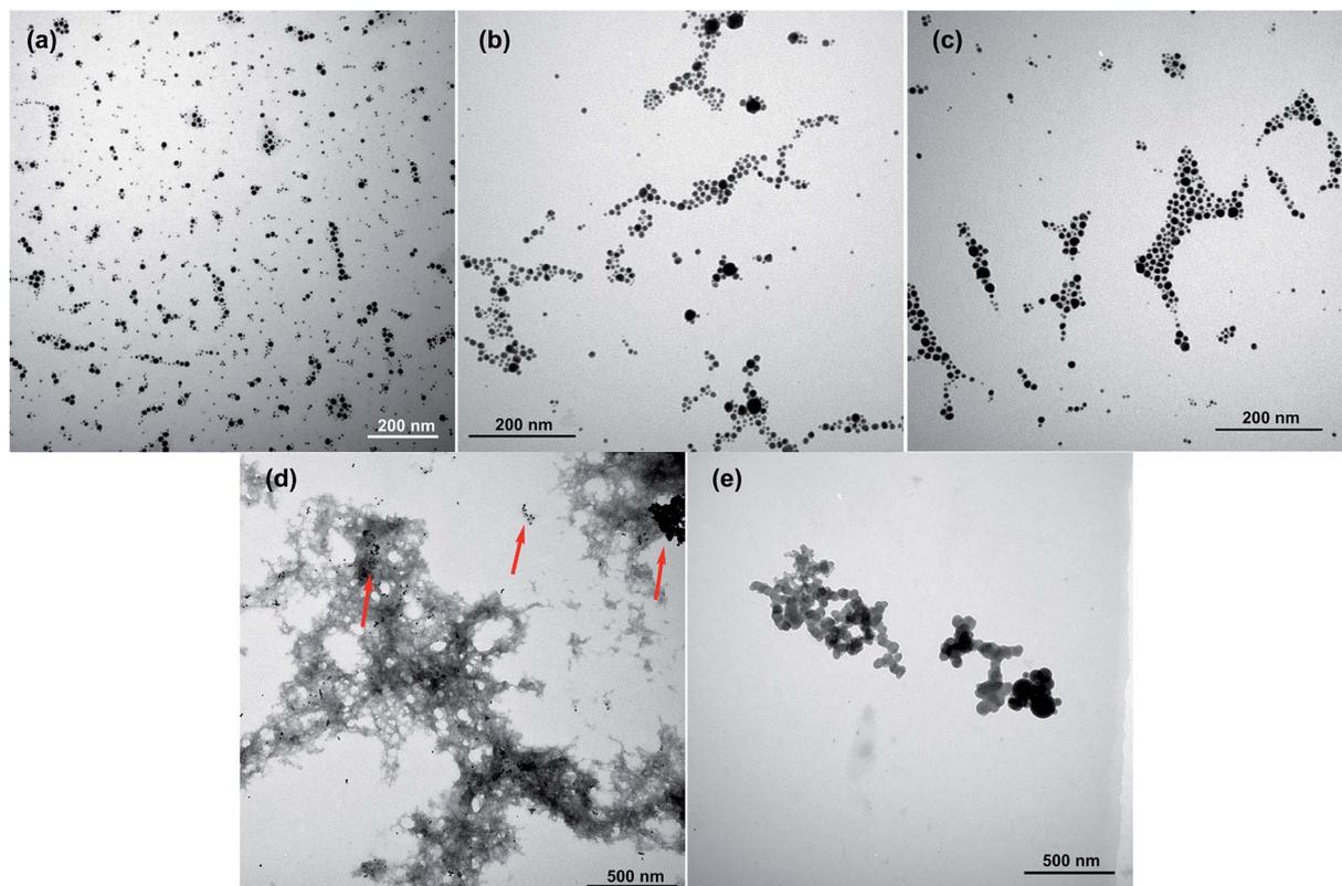
Fig. 6 The TEM images of GY-14@Au NPs with (a) 0.5 mM, (b) 5 mM and (c) 10 mM  $\text{Ca}^{2+}$  ions; (d) GY-14 + cit@Au NPs with 10 mM  $\text{Ca}^{2+}$  ions and (e) GY-14 with 10 mM  $\text{Ca}^{2+}$  ions.
