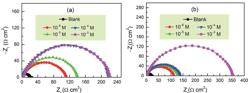
Fig. 2 Nyquist plots for carbon steel in 1 M HCl in the absence and presence of (a) CPT and (b) MPT at different concentration at 303 K.
