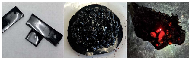
Fig. 1 Shaped materials can be fabricated from TTS_x thermosets by curing the comonomer solution at 150 °C in a mould or on a substrate, as illustrated by the rectangular prismatic brick (left) and patterned disc-shaped item (centre). A backlit sample of TTS_x (right) better illustrates the red colour and transparency of the material.
