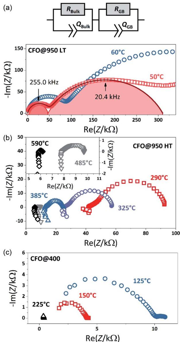
Fig. 3 (a) Nyquist plot of the impedance spectrum of CFO@950 measured in the temperature range between  $-45$  and 70 °C (just 60 and 50 °C shown) and the equivalent circuit used to describe the data. Nyquist plot of the impedance spectrum of (b) CFO@950 measured between 290 and 590 °C, and (c) of CFO@400 measured between 125 and 225 °C.
