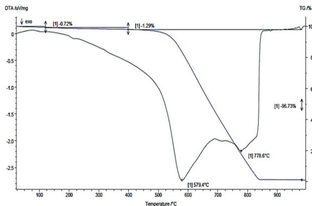
Fig. 7 TGA/DTG curves of pristine MWCNTs obtained under 120 mL min<sup>-1</sup> atmospheric air flow and 5 °C min<sup>-1</sup> heating rate.
