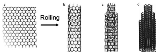
Fig. 1 Carbon nanotubes (CNT) composed of (a) sheet of graphene (b) single (SWCNT), (c) (DWCNT) double and (d) multiple layers (MWCNT), following Jackson, et al.<sup>17</sup>
