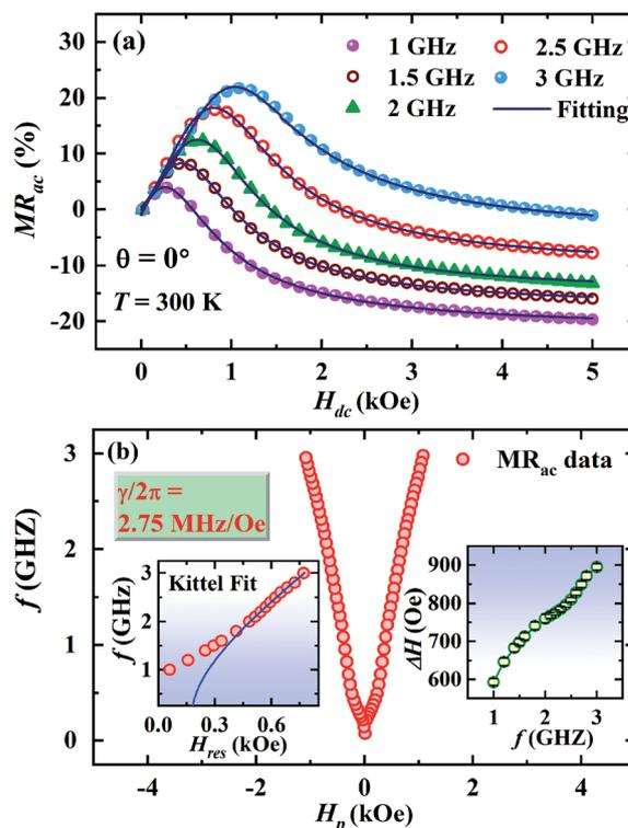
Fig. 6 (a) Fitting of  $\text{MR}_{\text{ac}}$  line shapes for  $\theta = 0^\circ$ . (b) Main panel: a plot of frequency ( $f$ ) as a function of the dc magnetic field ( $H_{\text{p}}$ ) at which the ac MR shows a peak, left inset shows Kittel-fit to the plot of  $f$  vs. resonance field ( $H_{\text{res}}$ ) extracted from the  $\text{MR}_{\text{ac}}$  data and right inset shows frequency dependence of linewidth ( $\Delta H$ ).
