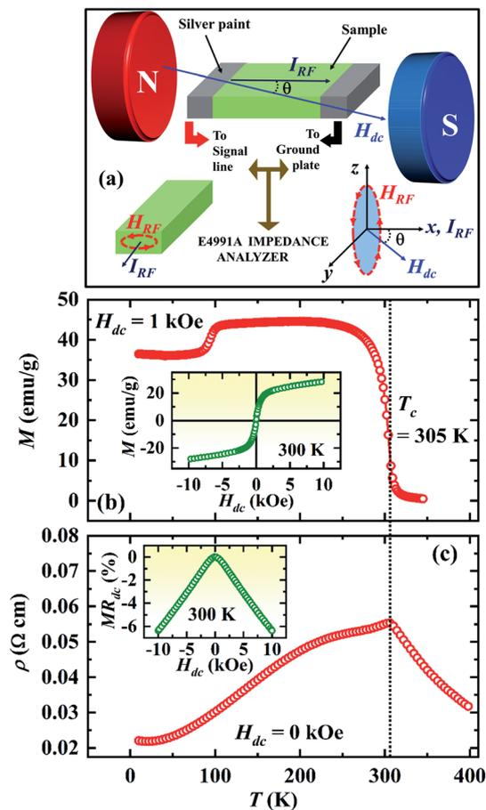
Fig. 1 (a) A schematic illustration of the broadband magnetoimpedance experimental configuration. (b) Temperature dependence of magnetization,  $M(T)$  of  $\text{Pr}_{0.6}\text{Sr}_{0.4}\text{MnO}_3$  in a magnetic field of  $H_{dc} = 1 \text{ kOe}$ , inset shows  $M(H)$  isotherm at 300 K (c) temperature dependence of four-probe dc resistivity of  $\text{Pr}_{0.6}\text{Sr}_{0.4}\text{MnO}_3$ , inset shows the dc magnetoresistance,  $\text{MR}_{dc}$  at 300 K.
