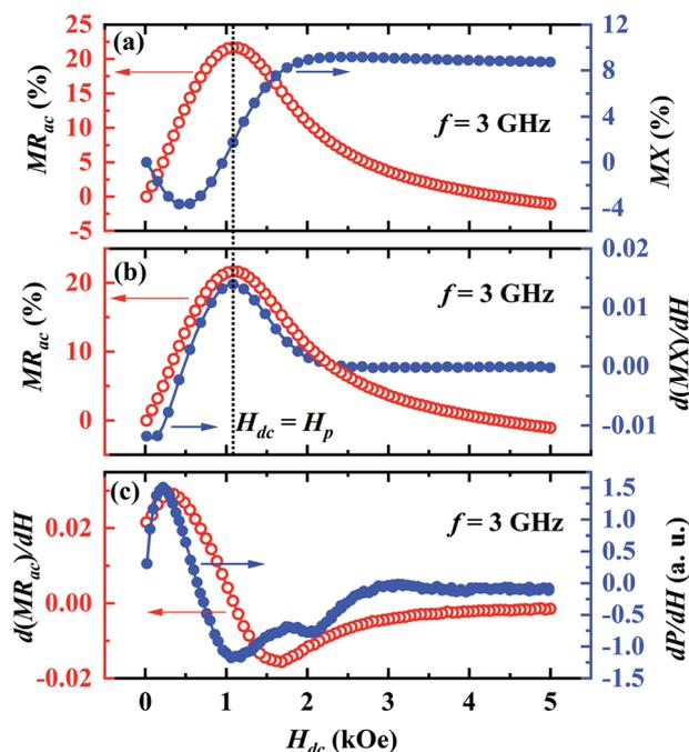
Fig. 5 (a)  $MR_{ac}$  on the left scale and MX on the right scale, (b)  $MR_{ac}$  on the left y scale and first derivative of the MX ( $d(MX)/dH$ ) on the right scale, (c) first derivative of the  $MR_{ac}$  ( $d(MR_{ac})/dH$ ) on the left y scale and  $dP/dH$  on the right scale for  $f = 3$  GHz at  $T = 300$  K.
