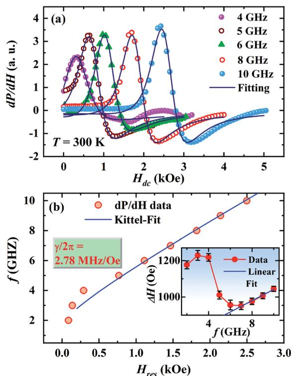
Fig. 7 (a) Fitting of  $dP/dH$  line shapes at  $T = 300 \text{ K}$  for different frequencies. (b) main panel shows the Kittel-fit to the plot of frequency ( $f$ ) vs. resonance field ( $H_{res}$ ) extracted from  $dP/dH$  data and the inset shows frequency dependence of  $\Delta H$  with a linear fit for  $f > 6 \text{ GHz}$ .
