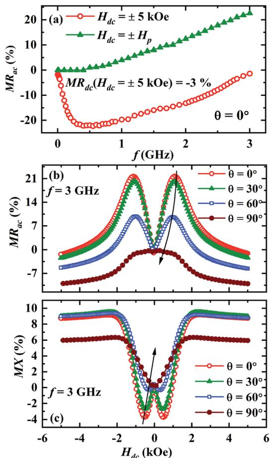
Fig. 3 (a) The ac MR as a function of frequency at room temperature for  $\theta = 0^\circ$ , magnetic field dependence of (b)  $MR_{ac}$  and (c) MX for  $\theta = 0^\circ, 30^\circ, 60^\circ$  and  $90^\circ$  at a fixed frequency  $f = 3$  GHz.
