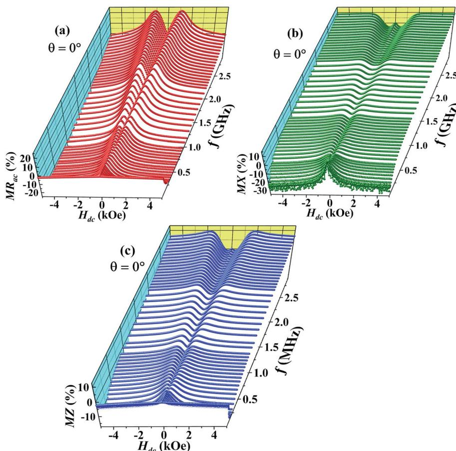
Fig. 2 Magnetic field dependence of (a) ac magnetoresistance ( $MR_{ac}$ ) (b) magnetoreactance (MX) and (c) magnetoimpedance (MZ) as a percentage change at  $T = 300$  K for  $\theta = 0^\circ$  for different frequencies of the ac current between  $f = 1$  MHz and 3 GHz.
