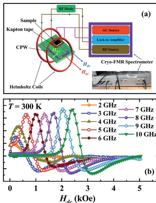
Fig. 4 (a) A schematic representation of the broadband FMR setup, (b) magnetic field dependence of the field derivative of the microwave power absorption ( $dP/dH$ ) at  $T = 300$  K at selected fixed frequencies of the microwave magnetic field ( $f = 2$  to 10 GHz).
