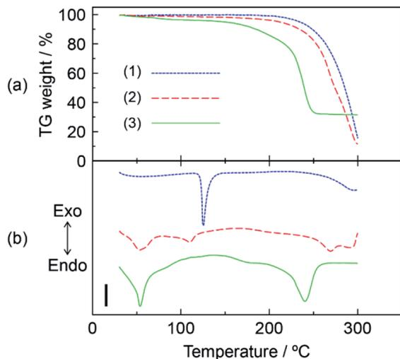
Fig. 1 TG (a) and DTA (b) curves of (1) DOT material, (2) DOT-40 mol% MDP composite material, and (3) MDP material. These measurements were done at the heating rate of 10 °C min<sup>-1</sup> under flowing dry-nitrogen. The TG-DTA measurements were normalized at 1 mg. Scale bar in (b) indicates 10 μV mg<sup>-1</sup>. Triplicate experiments gave similar results.
