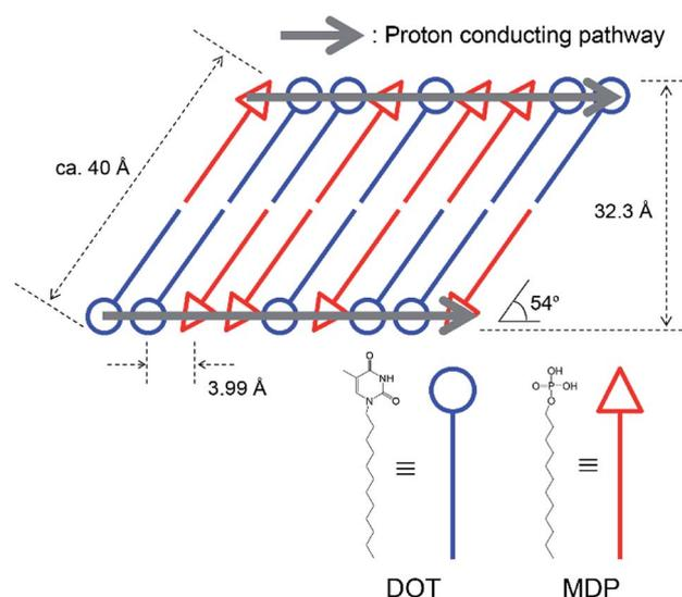
Scheme 3 Structural model with the proton conducting pathway of the DOT-MDP composite material. The distances between the molecules were estimated from the XRD measurements and the molecular modelling.
