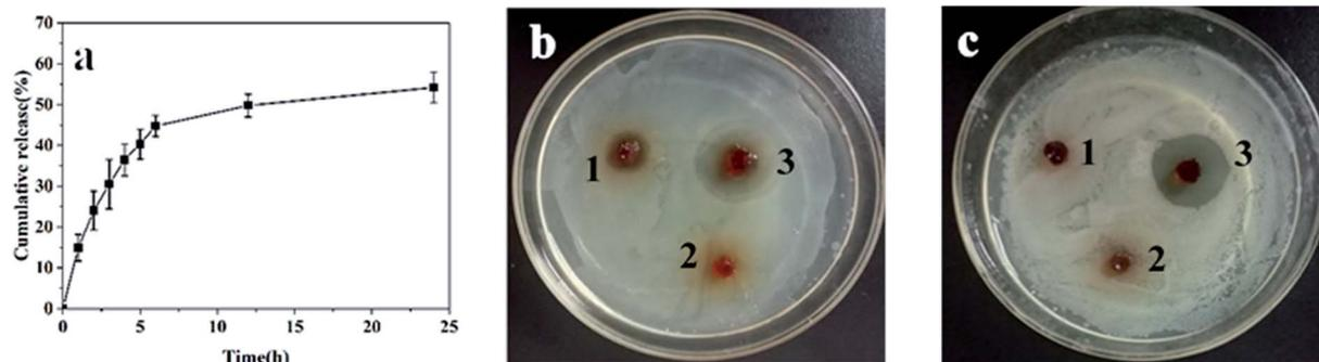
Fig. 5 (a) Release curve of levofloxacin from the CMC-GEL/OSA hydrogel. Inhibition zone of (b) *Escherichia coli* and (c) *Staphylococcus aureus*, sample 1, 2 and 3 were CMC/OSA gel, CMC-GEL/OSA gel and levofloxacin loaded CMC-GEL/OSA gel, respectively. The concentrations of CMC, GEL, OSA and levofloxacin were 5%, 20%, 15%, and 200 mg kg<sup>-1</sup>, respectively.
