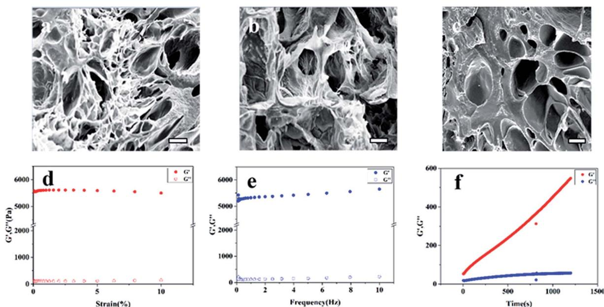
Fig. 4 SEM diagram of the cross-section of the hydrogels (scale bar, 100  $\mu$ m) (a) CMC/OSA, (b) GEL/OSA, (c) CMC-GEL/OSA. Rheological analysis of the CMC-GEL/OSA hydrogel (d) strain sweep (e) frequency sweep (f) time sweep. The concentration of CMC, GEL, and OSA was 5%, 20%, and 15%, respectively.
