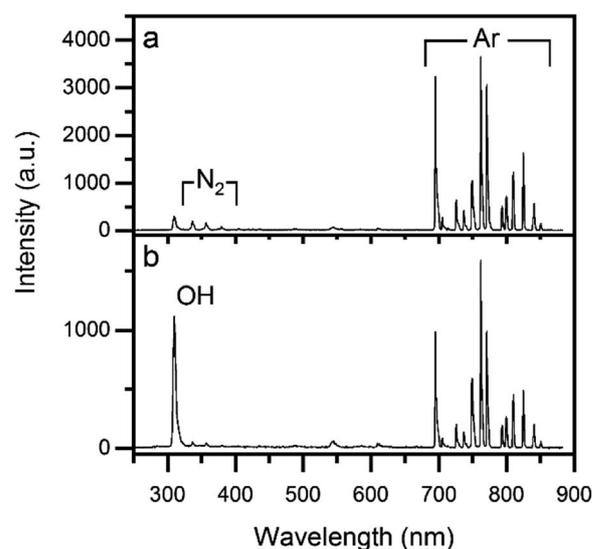
Fig. 2 OES spectra of (a) pure Ar plasma and (b) Ar/H<sub>2</sub>O plasma.
