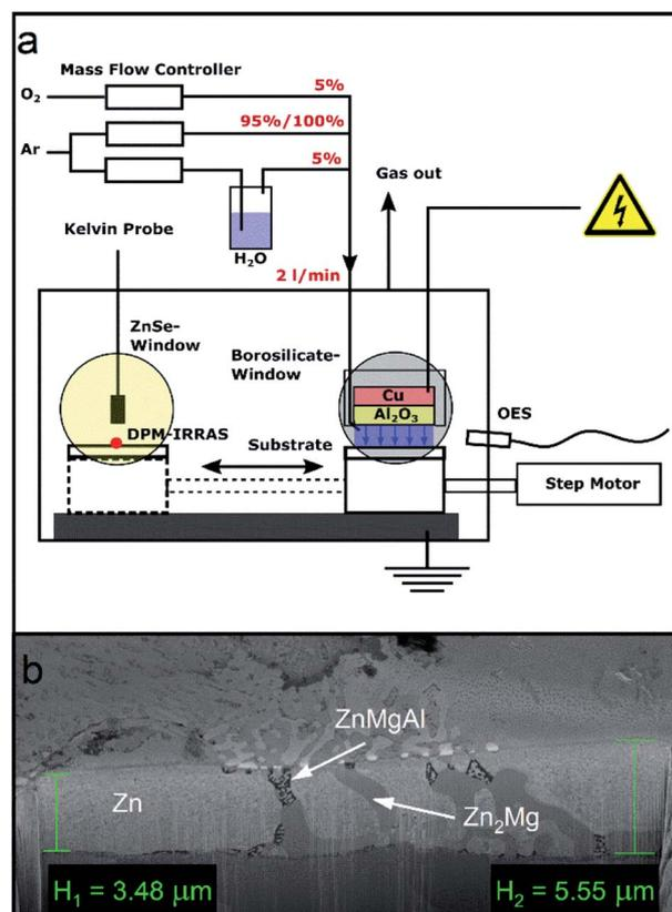
Fig. 1 (a) DBD plasma experimental setup used to treat the ZnMgAl surface and to investigate the plasma induced changes *in situ* with discrete polarized modulated FT-IRRAS and Kelvin probe. (b) SEM cross-section of the native ZnMgAl alloy layer onto steel.
