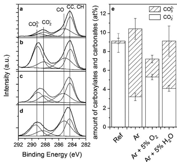
Fig. 4 Element spectra of C 1s before (a) and after the plasma treatment with Ar (b), Ar/O<sub>2</sub> (c) and Ar/H<sub>2</sub>O (d). Quantification of carboxylates and carbonates determined by XPS before and after the plasma treatments (e).
