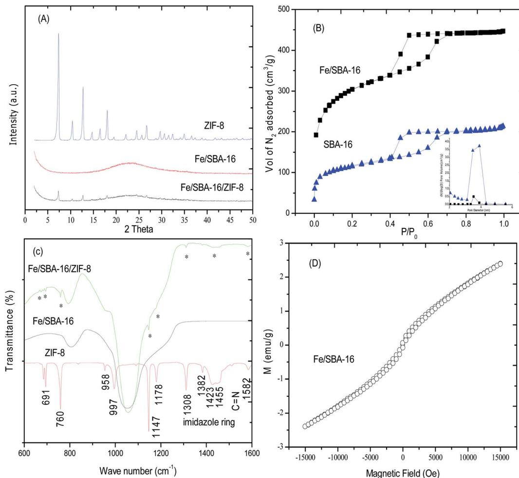
Fig. 3 Textural characterization of ZIF-8, Fe/S-16 and Fe/S-16/ZIF-8 using (A) X-ray diffraction (XRD), (B)  $N_2$ -adsorption isotherms, (C) Fourier-transformed infrared (FTIR) spectra and (D) vibrating sample magnetometry (VSM) analysis.
