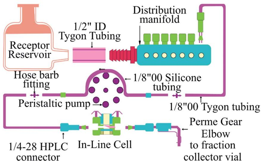
**Scheme 1** Schematic diagram of automated diffusion cell system equipped with flow type Franz cell.
