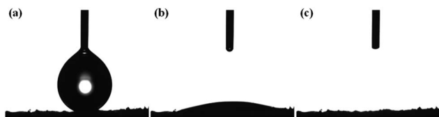
Fig. 4 (a) Initial, (b) transition, and (c) final stage of the quick absorption and percolation of water droplet by the prepared GO/Na-ALG scaffold.
