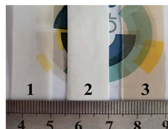
Fig. 2 Optical images of (1) pure PFSA (control), (2) SH–SiO 2 /PFSA, and (3) HSO 3 –SiO 2 /PFSA films.
