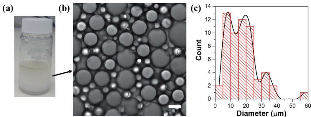
Fig. 5 (a) Prior modification of Aerosil® 300 silica nanoparticles with APTES ( $\text{SiO}_2$ -APTES) leads to an inefficient emulsification of 1 : 1 v/v toluene in water, with creaming occurring after preparation. (b) Confocal microscopy image of the emulsified volume of toluene in water (middle part of the vial presented in (a), arrow), stabilized by 1% w/v  $\text{SiO}_2$ -APTES nanoparticles (scale bar 20  $\mu\text{m}$ ). (c) Droplet size distribution of the o/w emulsion shown in (b).
