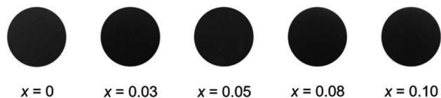
Fig. 5 Photographs of the \text{Ca}_2\text{Mn}_{0.85-x}\text{Ti}_{0.15}\text{Zn}_x\text{O}_{4-x} ( 0 \leq x \leq 0.10 ) pigments.
