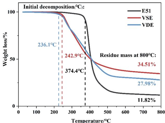
Fig. 4 TG and DTG curves for cured DGEBA, VSE and VDE from 40 °C to 200 °C under N<sub>2</sub>, purge gas velocity is 100 ml min<sup>-1</sup>.
