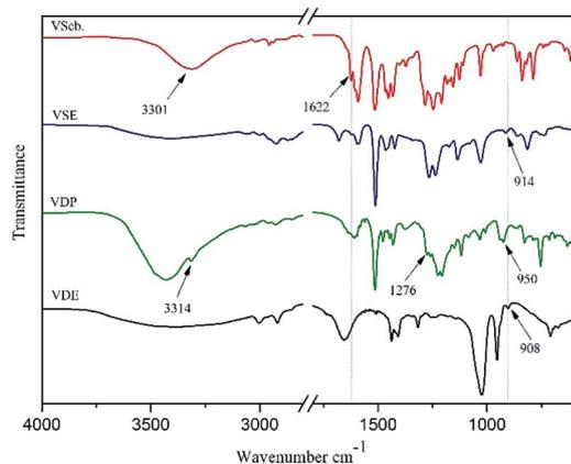
Fig. 1 FTIR spectra of Vscb, VSE, VDP and VDE scanned from 500–4000 cm<sup>-1</sup>.
