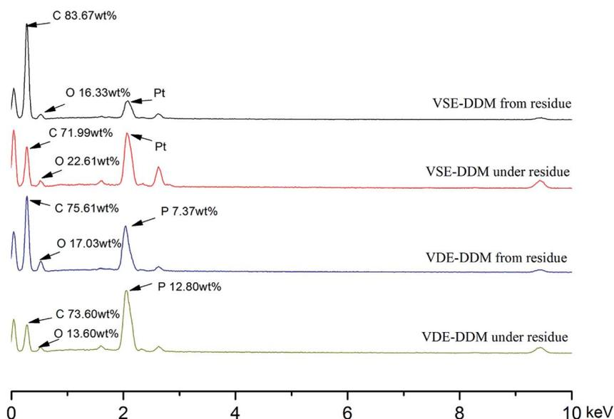
Fig. 10 EDS spectrum of char layer from the residue and the adjacent surface below the frontmost char layer.
