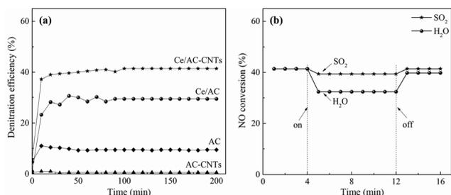
Fig. 3 Variation of (a) NO conversion of AC, AC-CNTs, Ce/AC and Ce/AC-CNTs, and (b) SO<sub>2</sub> tolerance and water-resistance of Ce/AC-CNTs over time. Reaction conditions: [NO] = 500 ppm, [NH<sub>3</sub>/NO] = 1.1, [O<sub>2</sub>] = 5 vol%, [SO<sub>2</sub>] = 50 ppm (when used), [H<sub>2</sub>O] = 10 vol% (when used), N<sub>2</sub> balance, reaction temperature = 150 °C and GHSV = 50 000 h<sup>-1</sup>.
