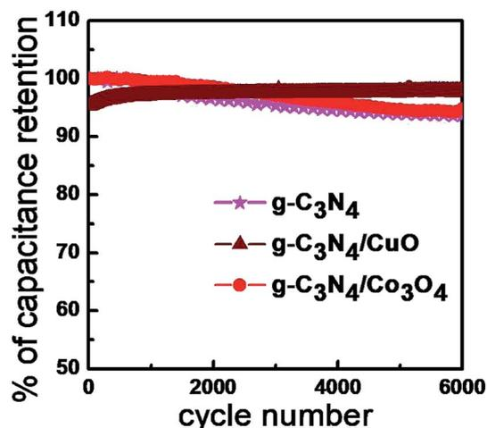
Fig. 8 Cycling stability curve of the supercapacitors at a constant current density of  $5 \text{ A g}^{-1}$ .
