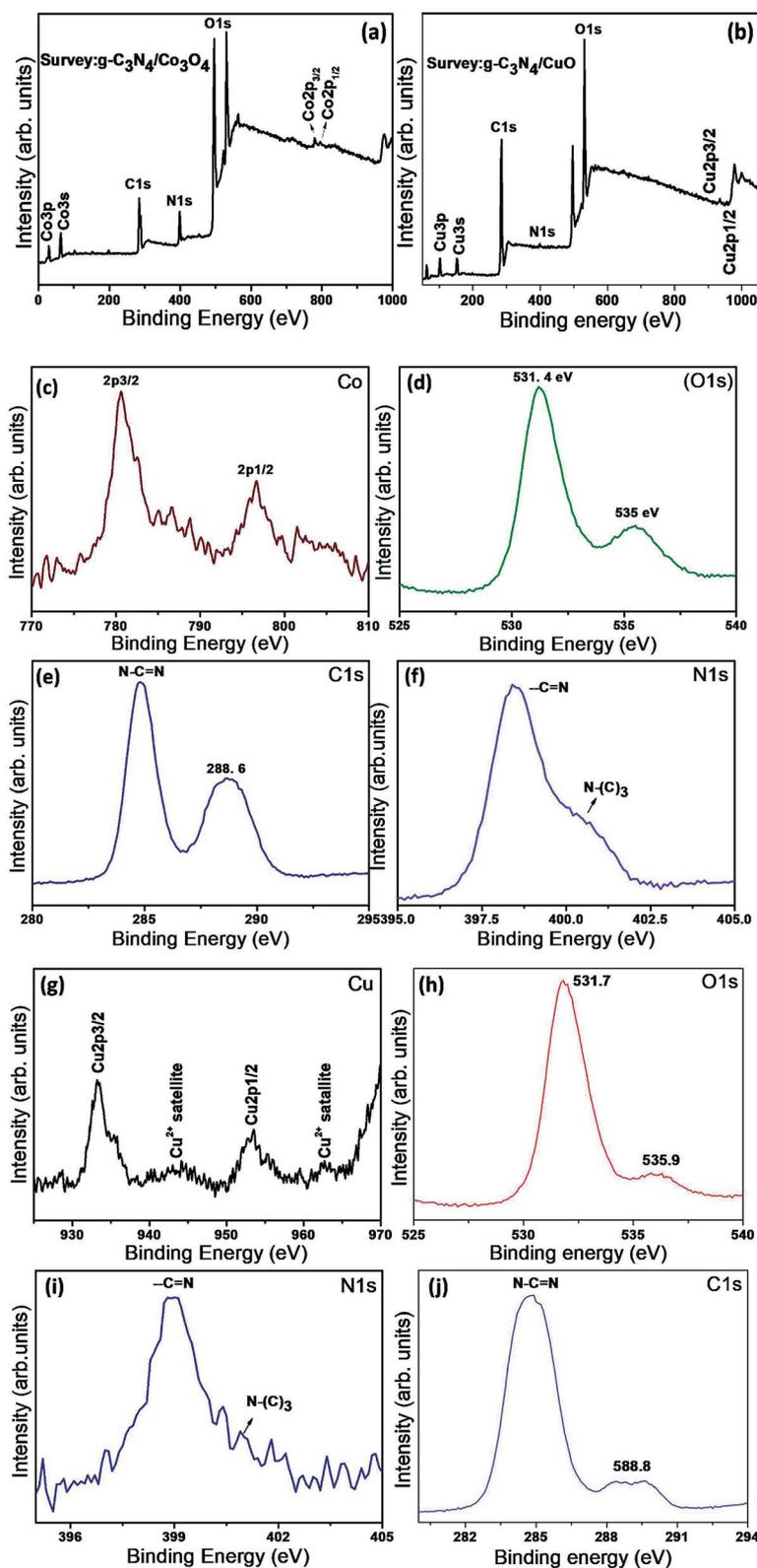
Fig. 3 Survey XPS spectrum of (a)  $g\text{-C}_3\text{N}_4/\text{Co}_3\text{O}_4$  and (b)  $g\text{-C}_3\text{N}_4/\text{CuO}$ . High resolution spectra of (c) Co 2p, (d) O 1s, (e) C 1s and (f) N 1s in  $g\text{-C}_3\text{N}_4/\text{Co}_3\text{O}_4$ . High resolution spectra of (g) Cu 2p (h) O 1s (i) N 1s and (j) C 1s.
