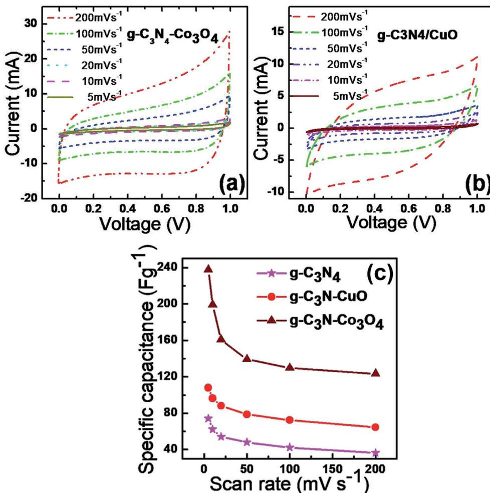
Fig. 6 Cyclic voltammograms of (a)  $g\text{-C}_3\text{N}_4/\text{Co}_3\text{O}_4$  and (b)  $g\text{-C}_3\text{N}_4/\text{CuO}$  at different scan rates. (c) Variation of specific capacitance of  $g\text{-C}_3\text{N}_4$ ,  $g\text{-C}_3\text{N}_4/\text{CuO}$  and  $g\text{-C}_3\text{N}_4/\text{Co}_3\text{O}_4$  with scan rate.
