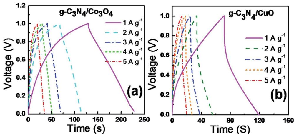
Fig. 7 GCD curves of (a)  $g\text{-C}_3\text{N}_4/\text{Co}_3\text{O}_4$  and (b)  $g\text{-C}_3\text{N}_4/\text{CuO}$  based supercapacitors at a constant current density of  $1 \text{ A g}^{-1}$  in  $2 \text{ M KOH}$  electrolyte.
