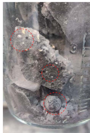
Fig. 6 Photo showing the dark sludge phase formed at the bottom of the salt after chemical purification of Mg. The excess Mg droplets are circled in red.
