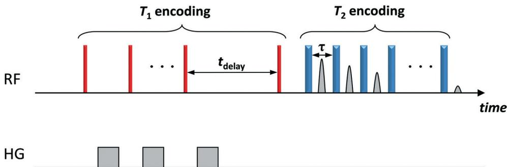
**Fig. 1** Two-dimensional  $T_1$ - $T_2$  NMR pulse sequence. The thin (red) and thick (blue) vertical bars represent  $90^\circ$  and  $180^\circ$  radiofrequency (RF) pulses, respectively.  $T_1$  relaxation is encoded in the variable time  $t_{\text{delay}}$ .  $T_2$  relaxation is encoded in the train of  $n$   $180^\circ$  pulses. A single data point is acquired at the centre of each echo time,  $\tau$ . The grey bars (HG) represent homospoil magnetic field gradients.
