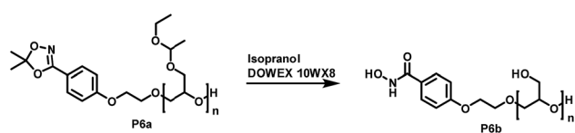
Scheme 6 Reaction scheme for cleavage of the protecting group in HAA-PEEGE releasing both the hydroxyl groups as well as the hydroxamic acid moiety.
