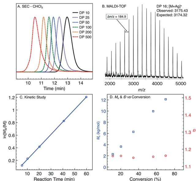
Fig. 2 (A) Size-exclusion chromatograms of  $P1_{\text{ROMP}}$  targeting different DPs. (B) MALDI-TOF-MS spectrum of  $P1_{\text{ROMP}}$ . (C) First-order kinetic plot for **1** targeting DP 100. (D)  $M_n$ -conversion correlation (blue) and  $D$ -conversion correlation (red).
