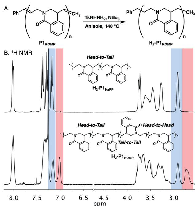
Fig. 4 (A). Reduction of **P1**<sub>ROMP</sub> to generate saturated polymer **H2-P1**<sub>ROMP</sub>. (B) Stacked <sup>1</sup>H NMR spectra and microstructures of **H2-P1**<sub>HaRP</sub> and **H2-P1**<sub>ROMP</sub>.
