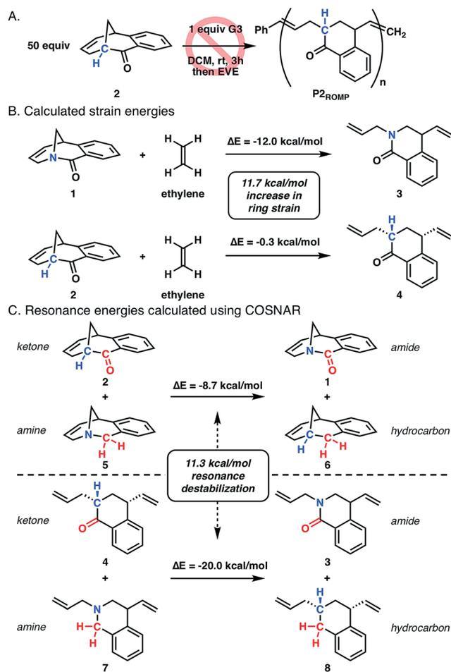
Fig. 3 (A) Attempted ROMP of ketone **2**. (B) Calculated ring strain energies of twisted amide **1** and ketone **2** from isodesmic ring-opening reaction with ethylene. (C) Resonance energies of amide **1** and **3** determined by COSNAR method (B3LYP-D3MBJ/6-311++G(d,p)).
