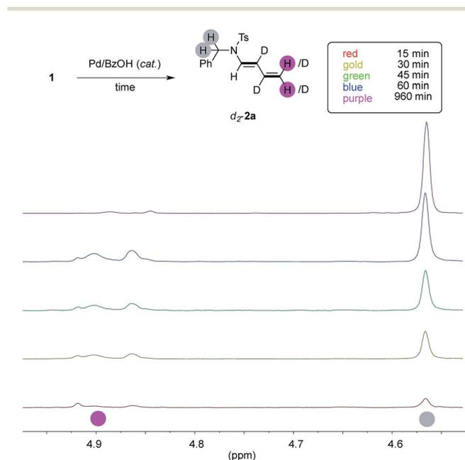
Fig. 3 Key  $^1\text{H}$ -NMR resonances through time.
