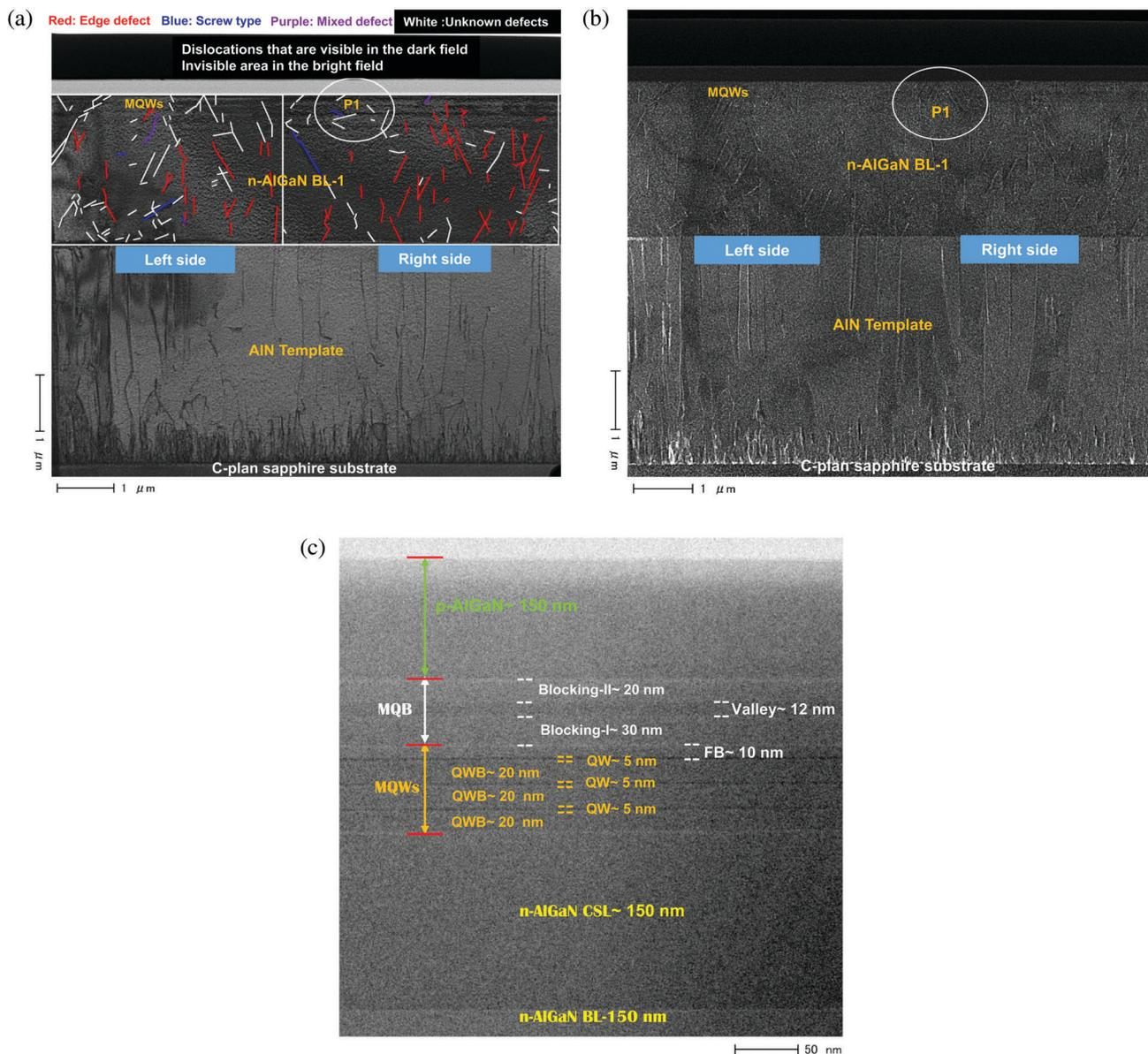
Fig. 4 (a) Cross-sectional HAADF-STEM images cut in the (10–10) zone axis tilted to  $g = (0002)$  showing the screw type dislocations, (b) cross-sectional TEM images cut in the (10–10) zone axis tilted to the  $g/3g$ ,  $g = (10-20)$  zone axis showing the edge and mixed type dislocations (sample-A), and (c) magnified annular bright-field (ABF)-STEM images of point area "P1" taken from Fig. 3(a) are shown to show the approximate thickness of the device structure.
