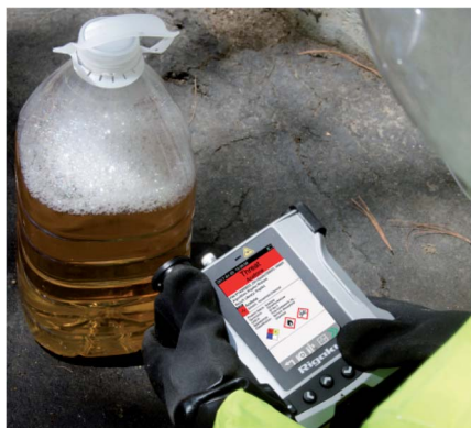
Fig. 4 Analysis of liquid inside a plastic container using a Raman analyser (image reproduced with the permission of SciMed/Rigaku).
