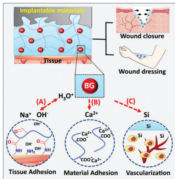
Fig. 12 Dual-adhesive and bioactive bioglass (BG)/oxidized sodium alginate (OSA) hydrogels. (A) The rapid ion exchange on the BG surface makes an alkaline environment to promote imine linkage formation between the tissues and the hydrogel. (B) The BG promotes adhesion between the hydrogel and materials via chelation between the carboxyl groups and \text{Ca}^{2+} released from BG. (C) The released Si ions promote vascularization in the wound area. Reprinted with permission from ref. 135. Copyright 2019, Springer Nature.
