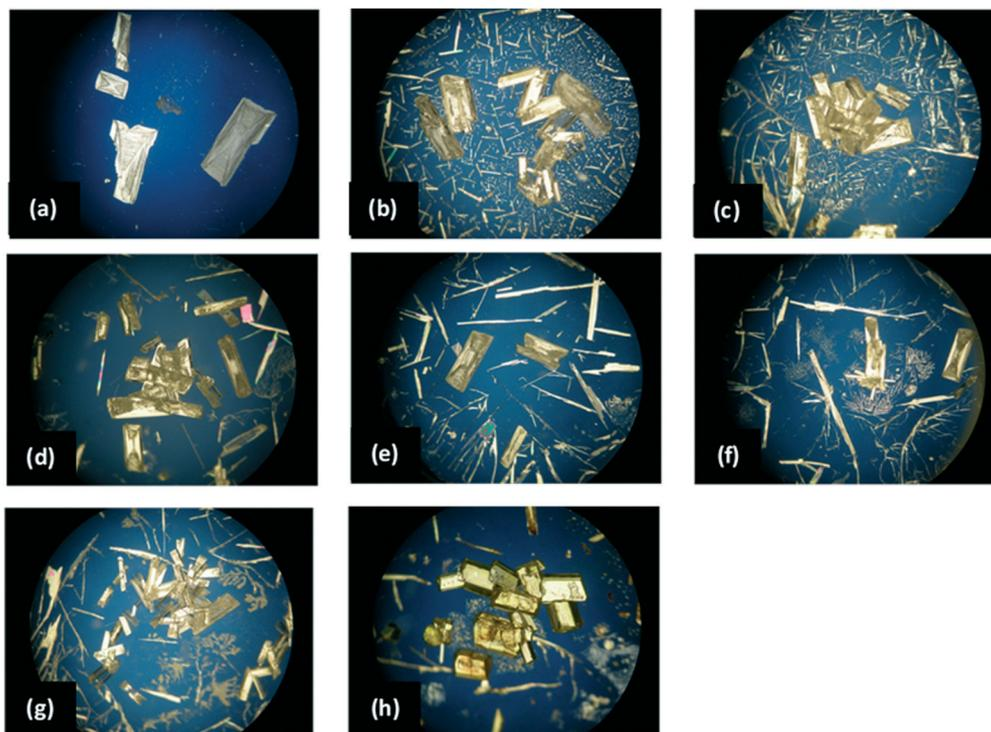
**Fig. 10** The morphology of IZN crystals from IPA observed in the presence of additives. (a) Absence of additive, (b) 3-cyanobenzoic acid, (c) 4-cyanobenzoic acid, (d) 3-hydroxybenzoic acid, (e) isonicotinamide, (f) nicotinamide, (g) 3,4-dihydroxybenzoic acid and (h) 3,4-dinitrobenzoic acid.
