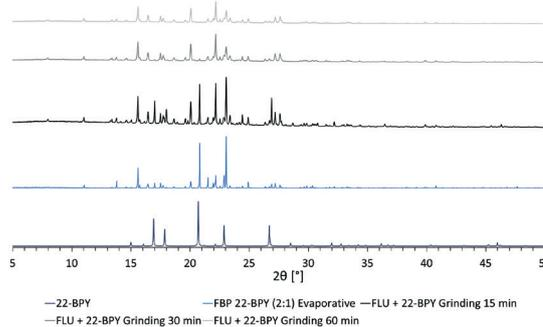
**Fig. 8** Formation of near-pure FLU 22-BPY (2:1) co-crystal by mechanochemical crystallisation methods with extended grinding times. Peaks associated with the 22-BPY starting material are most obvious and are seen to decrease in intensity as grinding time increases, with no evidence of starting material after 60 min.
