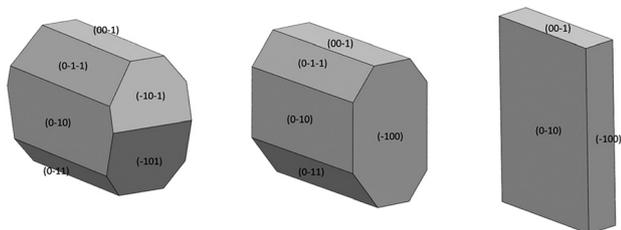
**Fig. 11** Crystal faces assigned by experimental face-indexing of IZN single crystals from additive screening studies. Left: IZN crystallised from propan-2-ol in the presence of 1% 3-hydroxybenzoic acid. Centre: IZN crystallised from propan-2-ol in the presence of 1% 3,4-dinitrobenzoic acid. Right: IZN crystallised from propan-2-ol in the absence of any additives.
