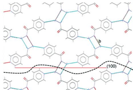
**Fig. 12** Overlay of the (100) plane (red line) with the underlying bulk IZN crystal structure in Mercury. “*b*” highlights discrete NH $\cdots$ N intermolecular hydrogen bonding interactions formed between adjacent hydrazine moieties. The black dashed line represents a hypothetical real surface termination for the (100) face, assuming only cleavage of intermolecular interactions.
