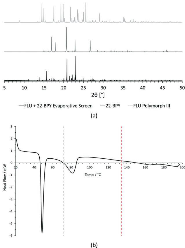
**Fig. 4** Initial analysis of [FLU + 22-BPY] evaporative crystallisation screening experiment. (a) Comparison of experimental PXRD data for sample with predicted PXRD patterns of starting materials (FLU polymorph III and 22-BPY) from CSD structure data. (b) Comparison of experimental DSC data for sample with starting material melting point data from literature (grey dashed line = 22-BPY melting point, red dashed line = FLU melting point).
