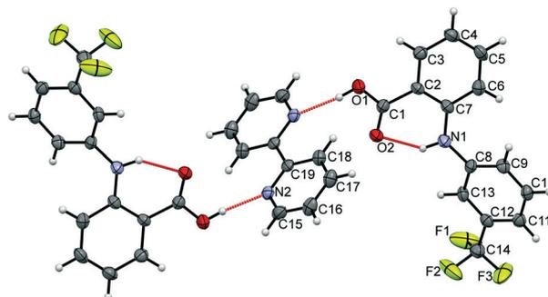
**Fig. 6** Single crystal X-ray structure of FLU 22-BPY (2:1) co-crystal, showing the atomic connectivity with ellipsoids shown at 50% probability. The CF<sub>3</sub> moiety is disordered and is modelled over two positions, though the second component is omitted here for clarity. Labelled atoms are included in the asymmetric unit, with the remaining structure is generated by symmetry. Red dashed lines indicate hydrogen bonding interactions.
