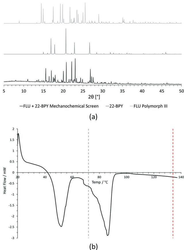
**Fig. 7** Initial analysis of [FLU + 22-BPY] mechanochemical crystallisation screening experiment. (a) Comparison of experimental PXRD data for 15 min ground sample with predicted PXRD patterns of starting materials (FLU polymorph III and 22-BPY) from CSD structure data. (b) Comparison of experimental DSC data for 15 min ground sample with starting material melting point data from literature (grey dashed line = 22-BPY melting point, red dashed line = FLU melting point).
