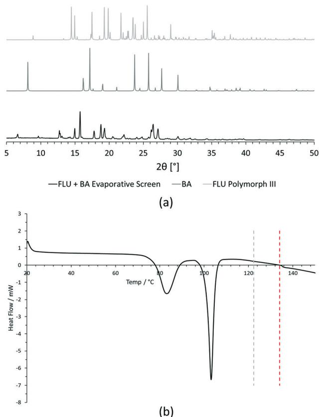
**Fig. 5** Initial analysis of [FLU + BA] evaporative crystallisation screening experiment. (a) Comparison of experimental PXRD data for sample with predicted PXRD patterns of starting materials (FLU polymorph III and BA) from CSD structure data. (b) Comparison of experimental DSC data for sample with starting material melting point data from literature (grey dashed line = BA melting point, red dashed line = FLU melting point).
