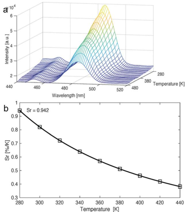
Fig. 36 (a) Emission map of Dy(acac)<sub>3</sub>-grafted TpBpy COF material recorded at 280–480 K. (b) Representation of the relative sensitivity values for the same compound at varying temperatures. Reprinted with permission from *Angew. Chem., Int. Ed.*, 2020, **59**, 2–11.
