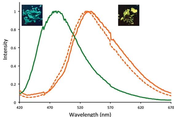
Fig. 12 Normalized emission spectra of Py-DBA-COF 1 (orange,  $\lambda_{\text{ex}} = 350$  nm), Py-DBA-COF 2 (green,  $\lambda_{\text{ex}} = 365$  nm), and Py-MV-DBA-COF (dashed orange,  $\lambda_{\text{ex}} = 350$  nm). Photographs of the fluorescent solids were taken using a hand-held UV-lamp at 365 nm. Reprinted with permission from *J. Am. Chem. Soc.* 2016, **138**, 10120–10123. Copyright 2016 American Chemical Society.
