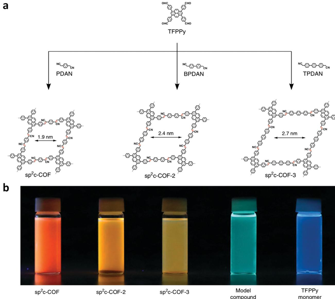
Fig. 4 (a) Design and structures of  $sp^2c$ -COFs from the condensation of TFPPy with PDAN, BPDAN, and TPDAN. (b) Images of  $sp^2c$ -COF,  $sp^2c$ -COF-2,  $sp^2c$ -COF-3, model compound, and TFPPy monomer dispersed in water under a UV lamp. Adapted with permission from *Nat. Commun.*, 2018, **9**, 4143.
