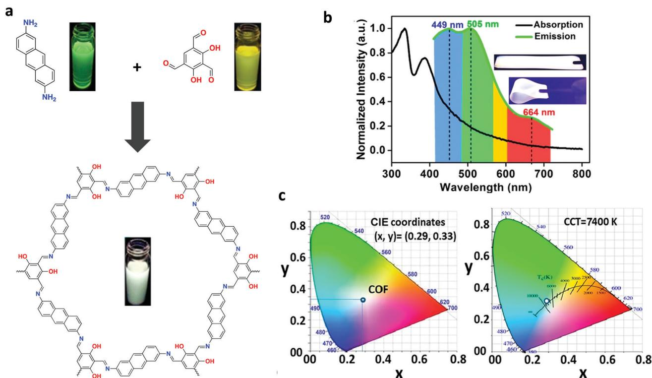
Fig. 34 (a) Synthesis of IISERP-COF7, including photographs of monomers and COF dispersed in NMP under a UV lamp. (b) Solid state absorption and emission spectra of COF@PMMA ( $\lambda_{\text{ex}} = 420$  nm), with inset photographs of COF@PMMA film under UV irradiation. (c) CIE coordinate and CCT diagram of COF film with a thickness of 2 mm. Adapted with permission from *J. Am. Chem. Soc.*, 2018, **140**, 13367–13374. Copyright 2018 American Chemical Society.
