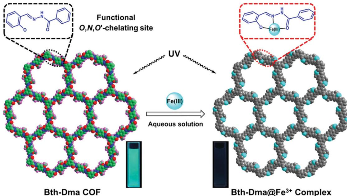
Fig. 21 Structure of Bth-Dma COF with and without the addition of  $\text{Fe}^{3+}$ . Inset photographs show the fluorescence quenching upon the formation of Bth-Dma@ $\text{Fe}^{3+}$  complex. Reprinted with permission from *ACS Appl. Mater. Interfaces*, 2019, **11**, 12830–12837. Copyright 2019 American Chemical Society.
