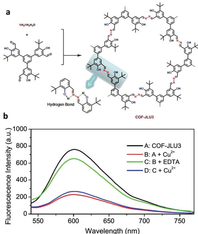
Fig. 20 (a) Synthesis of COF-JLU3 depicting the intramolecular hydrogen bonding. (b) Fluorescence spectra of COF-JLU3 demonstrating its effective reversible quenching by  $\text{Cu}^{2+}$  ions. Adapted from *Chem. Commun.*, 2016, 52, 6613, with permission from the Royal Society of Chemistry.
