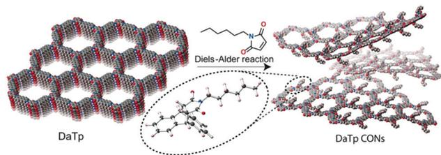
Fig. 3 Schematic representation of the chemical exfoliation process by layer planarity distortion with the Diels–Alder reaction. Inset: Energy-optimized structure of the cycloadduct of *N*-hexylmaleimide and anthracene. Reproduced from ref. 18 with permission from Wiley-VCH, copyright 2016.
