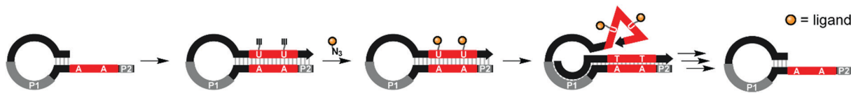
Fig. 5 SELMA (selection of modified aptamers) process: a library of hairpins is extended by polymerase which incorporates alkyne-modified uridines. Azide-modified ligands are conjugated through Cu-mediated click chemistry. Extension from primer site P1 ejects the ligand-decorated strand from the hairpin, allowing it to fold into a three-dimensional shape, which is screened against a target compound. Through multiple subsequent steps the starting hairpin can be regenerated for further selection rounds (ref. 21).
