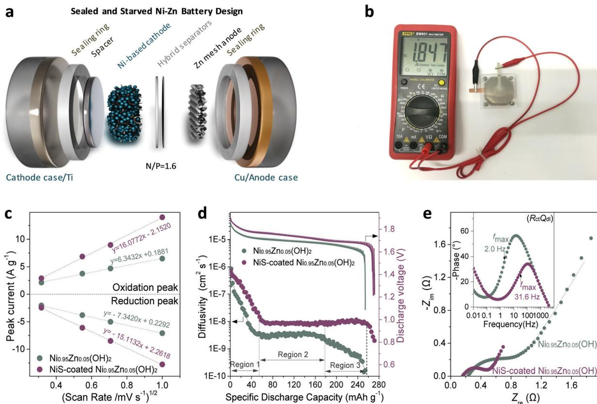
**Fig. 3** Kinetics analysis of the sealed and starved Ni–Zn design. (a) Schematic of the Ni–Zn demo battery design with high mass loading of  $80 \text{ mg cm}^{-2}$ . (b) Photograph of the designed cell and high open-circuit voltage of 1.847 V of the Ni–Zn cell. (c) Linear correlation between the peak current and the square root of the scan rate. (d) GITT curves and diffusivity versus DOD. (e) Nyquist plots. Inset: Bode plots of the  $(R_{\text{ct}}Q_{\text{dl}})$  parallel components.
