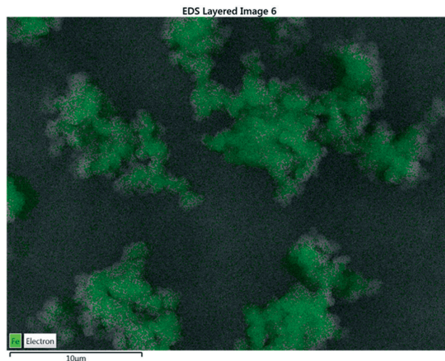
Fig. 3 EDS analysis of a sample of XFe-1.0.
