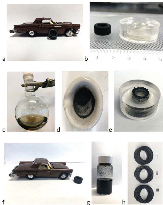
Fig. 4 (a) The right front tire was removed from a toy car. (b) A silicone mold of the tire. (c) Organic oil 8 was prepared by reduction of truck tire tread (Sailun, IR/NR) with hydrosilane 7 . (d) Silicone mold filled with 0.707 g 8 + 1 wt% BPO + 0.3010 g residual solid. (e) New tire after curing. (f) Tire replacement. (g) The residual solid during the preparation of 8 could be included in the pre-elastomer formulation. (h) Close up showing: (i) the original tire, (ii) tire made without additional inorganic excipients 13 , and (iii) tire including inorganic excipients.
